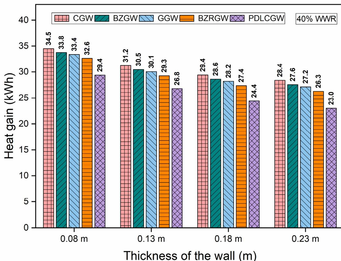
Figure 6. Heat gain in laterite rooms of different wall thicknesses of 40% WWR.
