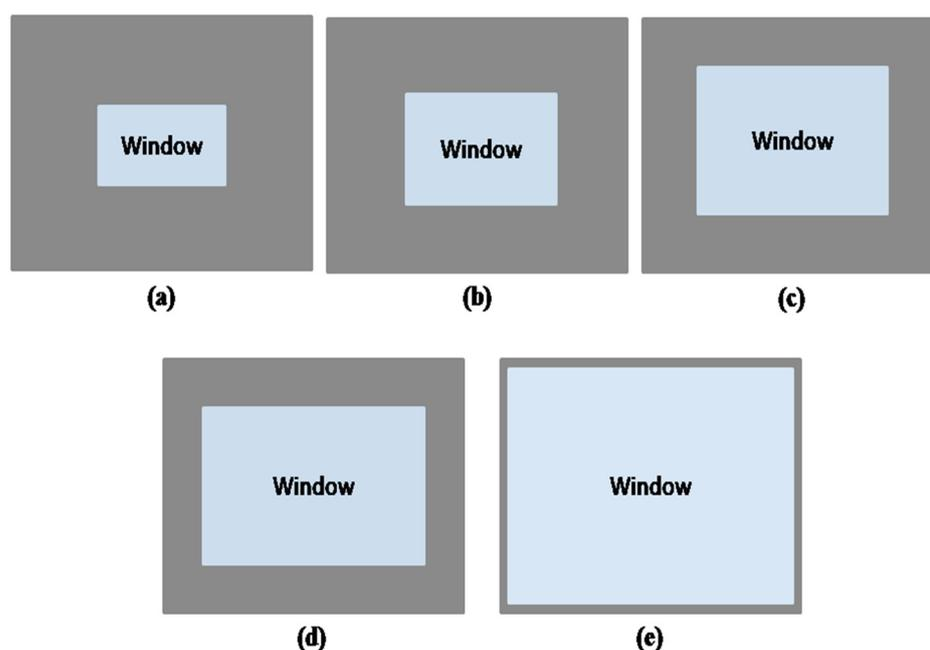
**Figure 4.** Building models: (a) with 20% WWR, (b) with 40% WWR, (c) with 60% WWR, (d) with 80% WWR, (e) with 100% WWR.
