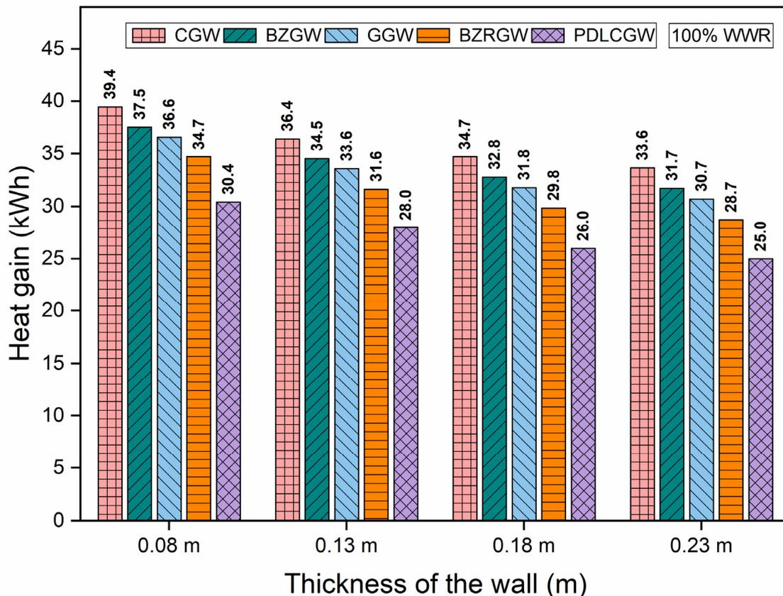
Figure 9. Heat gain in laterite rooms of different wall thicknesses of 100% WWR.
