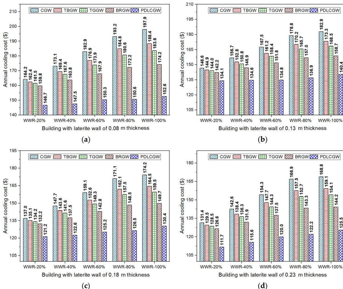
**Figure 10.** Influence of window glazing, its WWR, and wall thickness on cooling costs of laterite rooms (a) with 0.08 m thickness (b) with 0.13 m thickness (c) with 0.18 m thickness (d) with 0.23 m thickness.
