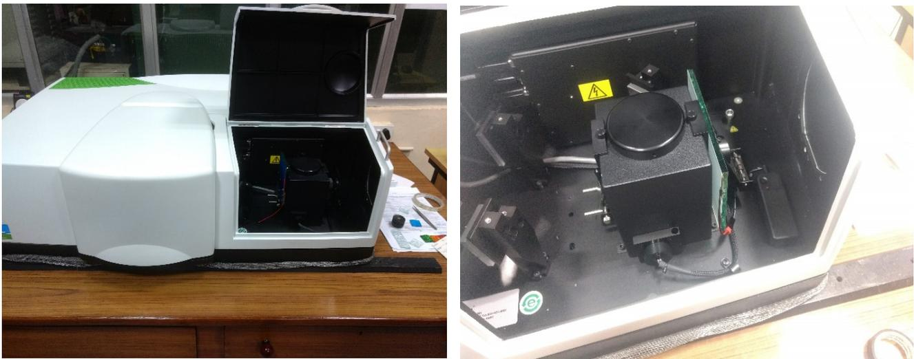
**Figure 1.** UV–VIS–NIR Perkin Elmer (Lambda 950) spectrophotometer.
