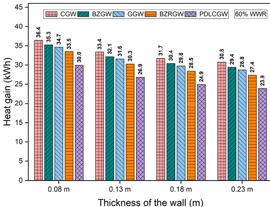
**Figure 7.** Heat gain in laterite rooms of different wall thicknesses of 60% WWR.
