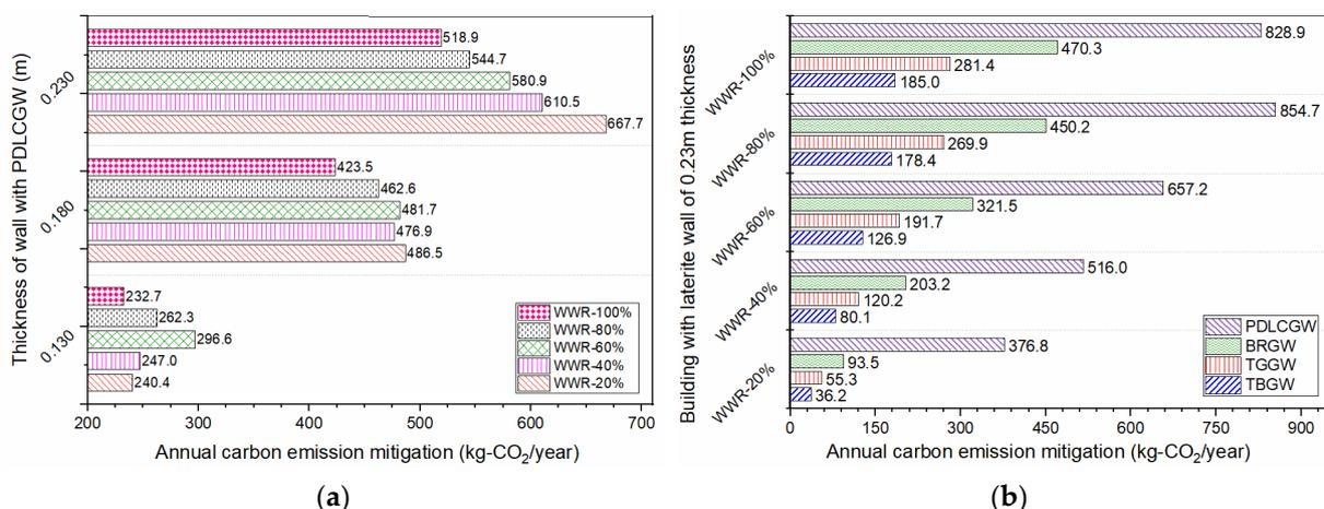
**Figure 12.** Influence of window glazing, its WWR, and wall thicknesses on carbon emission mitigation in laterite rooms (a) Effect of various thicknesses of laterite walls (b) Effect of WWR on various glazing systems.
