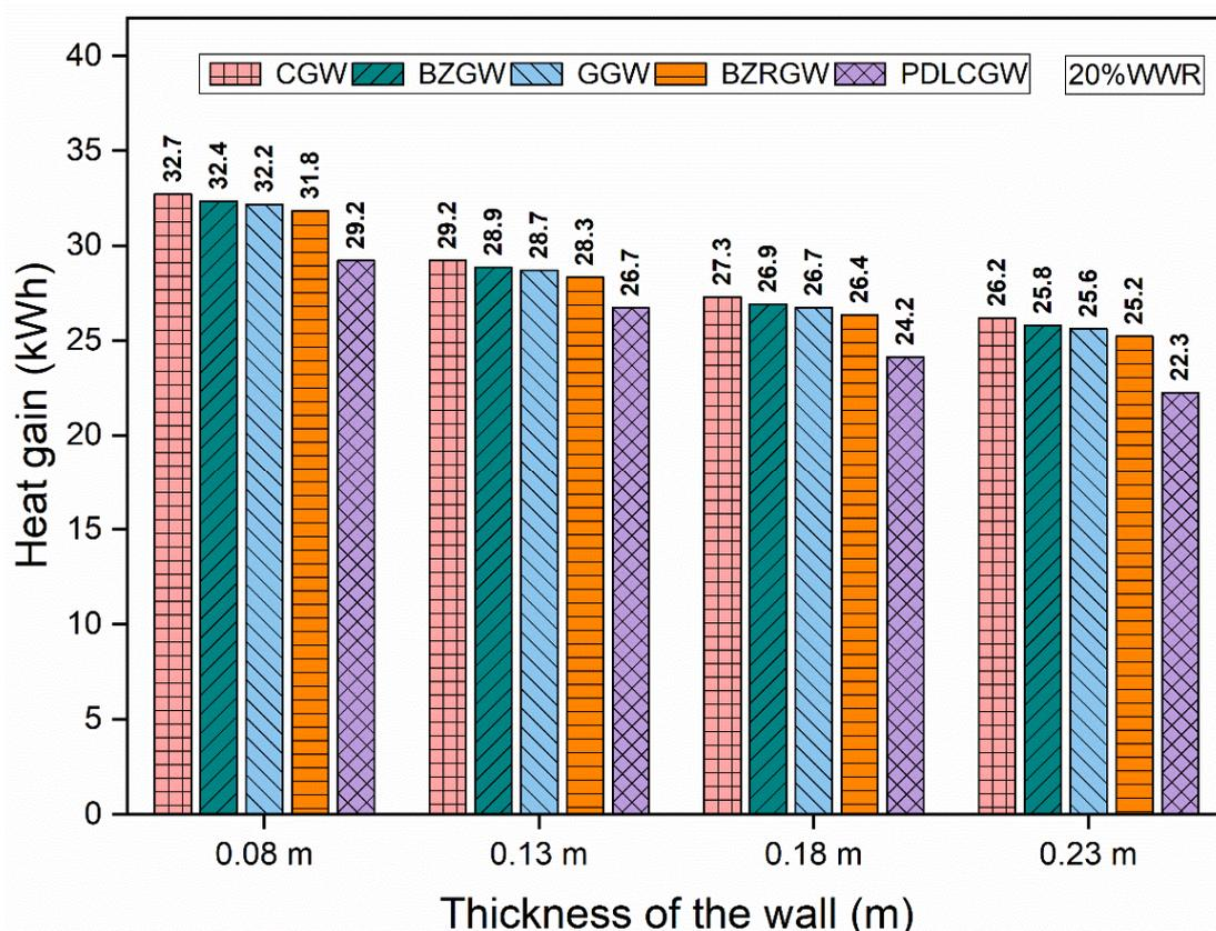
Figure 5. Heat gain in laterite rooms of different wall thicknesses of 20% WWR.
