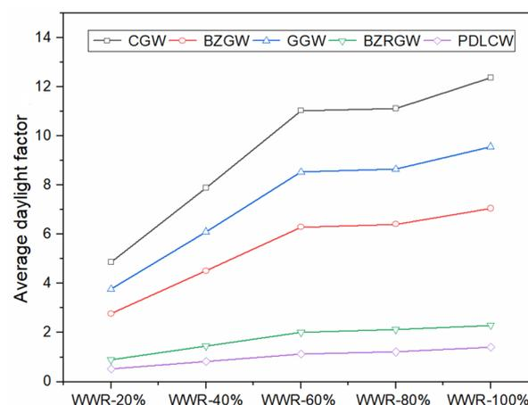
Figure 13. Influence of window glazing and its WWR on daylight factor in laterite rooms.
