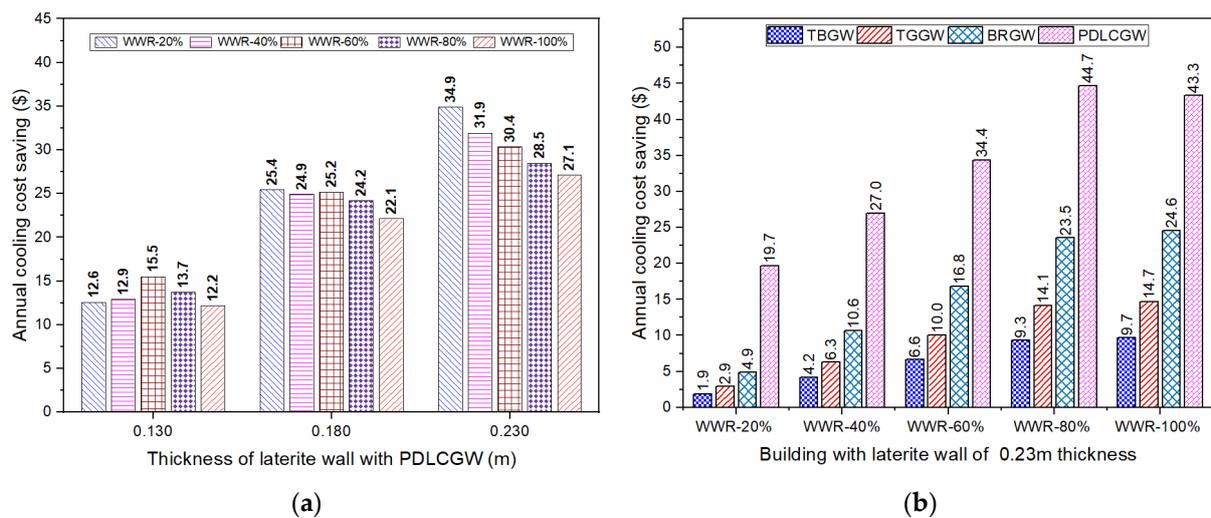
**Figure 11.** Influence of window glazing, its WWR, and wall thicknesses on annual cooling cost savings of laterite rooms (a) Effect of various thicknesses of laterite walls (b) Effect of WWR on various glazing systems.
