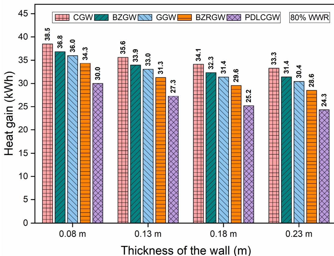
**Figure 8.** Heat gain in laterite rooms of different wall thicknesses of 80% WWR.
