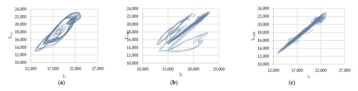
**Figure 5.** Attractors of the time series of load data in two-dimensional phase-spaces: (a)  $(Y_t, Y_{t-1})$ , (b)  $(Y_t, Y_{t-24})$ , and (c)  $(Y_t, Y_{t-168})$ .
