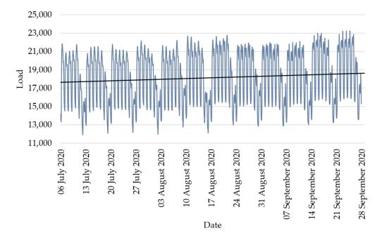
**Figure 3.** Hourly load data of the Polish Power System from 6 July 2020 to 27 September 2020 as a time series plot.
