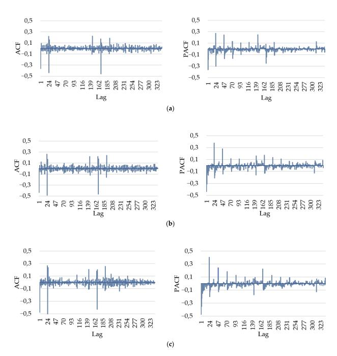
Figure 9. ACF and PACF of differentiated noise-disturbed time series: (a) NSR = 30%, (b) NSR = 100%, (c) NSR = 200%.
