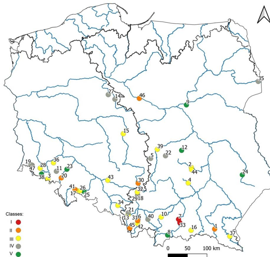
**Figure 4.** Classes of capacity changes (in %) in reservoirs of key importance for water management in Poland. Classes: I—large loss of capacity—over 30%, II—significant loss of capacity—10.1–30%,
