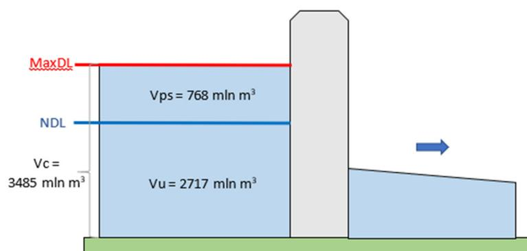
**Figure 2.** The current capacity of the analyzed 47 key reservoirs in Poland. Explanations: NDL (normal damming water level)—the highest level of the water table in normal conditions of use;
