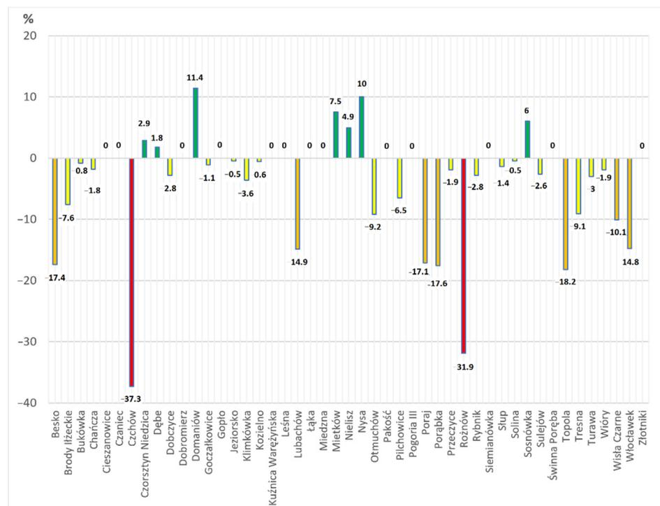
**Figure 3.** Structure of capacity change in reservoirs of key importance for water management in Poland. Classes: I—large loss of capacity—over 30% (red), II—significant loss of capacity—10.1–30% (orange), III—moderate loss of capacity—0.1–10% (yellow), IV—constant unchanged capacity (no color), V—increase in capacity (green).
