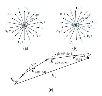
**Figure 6.** Star of slots and resultant phasors of target machines: (a) regular machine with  $\tau_t = 20^\circ$ ; (b) proposed machine with  $\tau_t = 18.1^\circ$ ; (c) resultant phasors of back-EMF.
