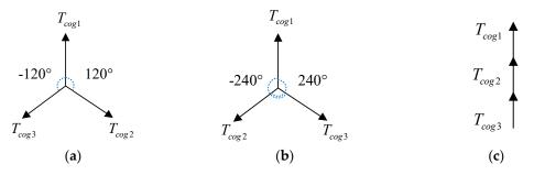
**Figure 9.** Cogging torque phasor diagram for equal angle: (a)  $N_{non}$  orders (b) 2  $N_{non}$  orders (c) 3  $N_{non}$  orders.
