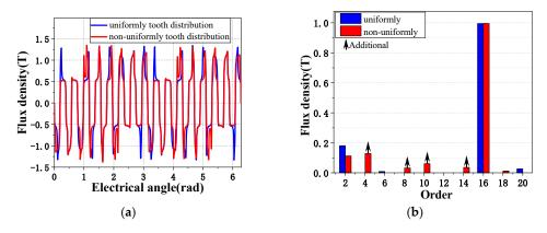
Figure 14. Comparison of airgap flux density by FEM: (a) flux density waveform; (b) spectra of FFT.
