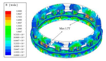
Figure 13. Flux density distribution of the 3D-FEM in on-load condition.
