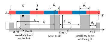
Figure 3. Expanded view of one tooth unit in non-uniform distribution.
