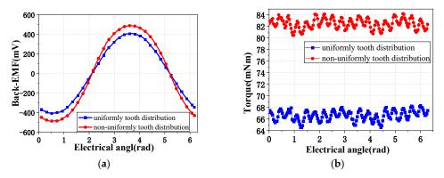
**Figure 15.** Comparison of performance at 50 rpm by FEM: (**a**) back-EMF; (**b**) electromagnetic torque with rated 0.4 A<sub>rms</sub> current.
