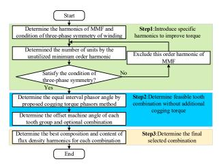
Figure 11. Design approach of non-uniform tooth distribution.
