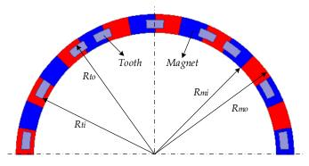
Figure 2. Top view of half proposed AFPMVM.
