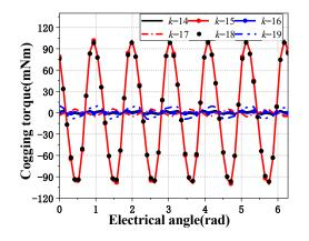
Figure 10. Cogging torque with different tooth pitch by FEM.
