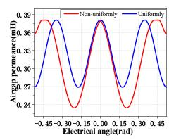
Figure 4. Analytical airgap permeance in one unit of two different tooth distribution topologies.
