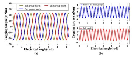
Figure 7. Cogging torque verification of proposed method by FEM: (a) each group (b) sum comparison.
