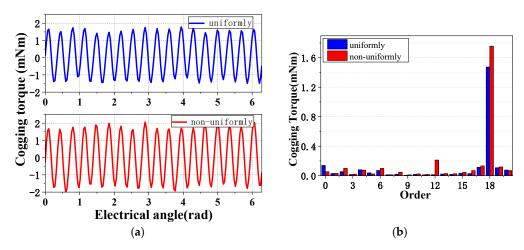
Figure 16. Cogging torque contrast by FEM. (a) Cogging torque. (b) Spectra of FFT.
