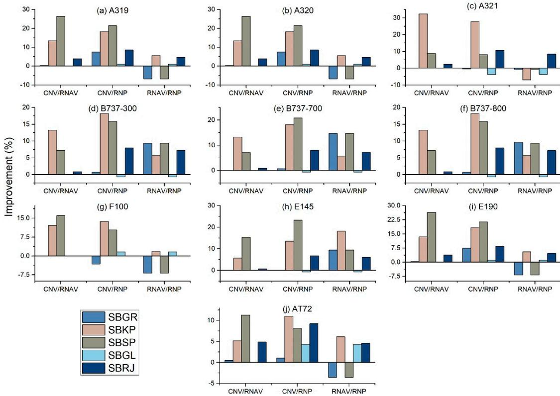
Figure 7. Case 1 approach; percentage improvement by aircraft. (a) A319; (b) A320; (c) A321; (d) B737-300; (e) B737-700; (f) B737-800; (g) F100; (h) E145; (i) E190; (j) AT72.
