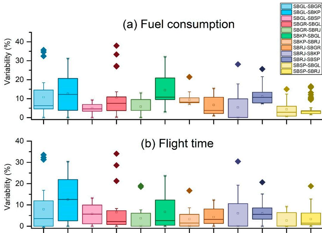
Figure 8. Gain variability for fuel consumption for each route due to air traffic interactions. (a) Fuel consumption; (b) Flight time.
