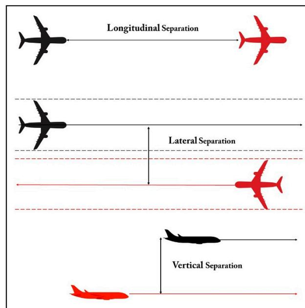
Figure 2. Longitudinal, lateral, and vertical separation. Source: The authors.
