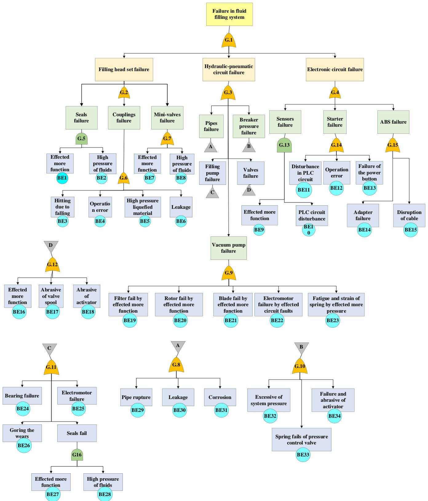
Figure 3. The FTA structure for the failures in a complex filling system in an Iranian automotive production line.
