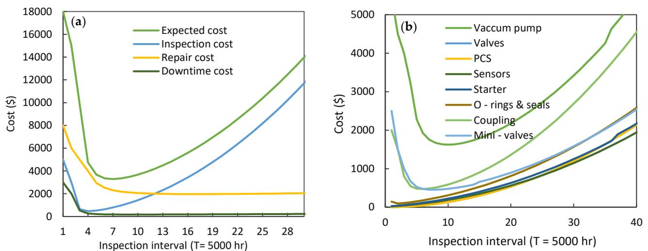
**Figure 10.** The optimal maintenance intervals for the (a) whole system and (b) critical components.
