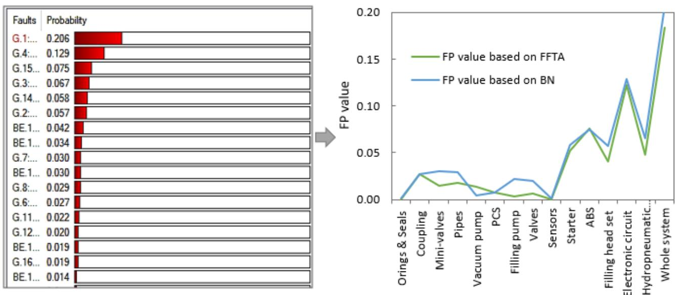
Figure 9. The comparison results of the FFTA and BN models.
