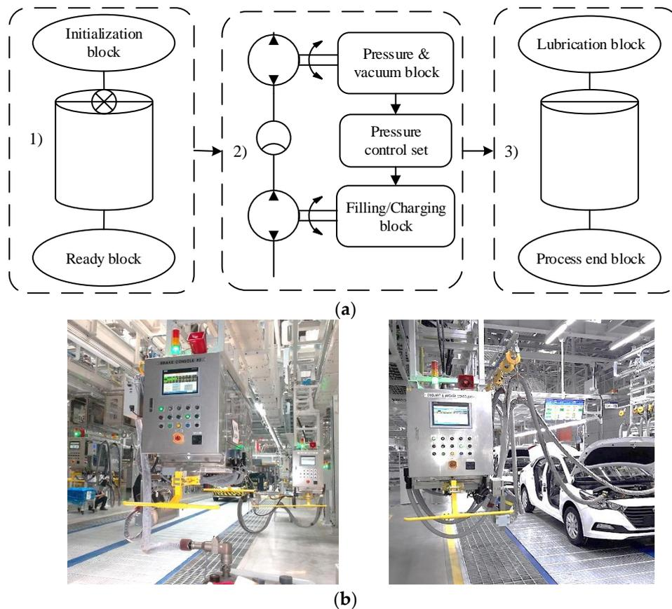
**Figure 1.** A filling system in an Iranian automotive assembly line. (a) Block diagram, and (b) functioning view.
