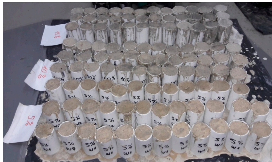
Figure 5. Regular samples filled with a backfill mixture with different cement contents.
