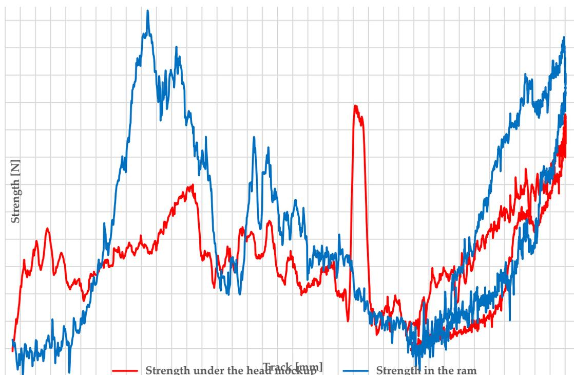
**Figure 8.** Force after impact on point P2—temperature of  $-80\text{ }^{\circ}\text{C}$ .
