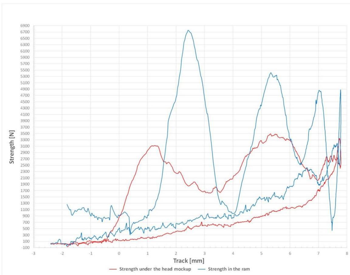
Figure 7. Force after impact on point P1—temperature of −80 °C.
