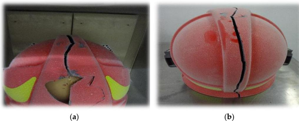
**Figure 9.** Helmet after testing at a temperature of  $-80\text{ }^{\circ}\text{C}$ : (a) after hitting point P1; (b) after hitting point P2.
