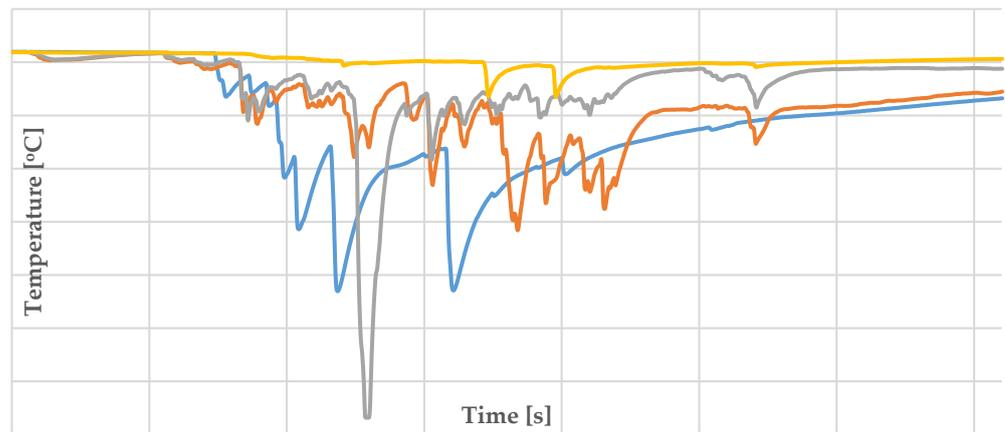
**Figure 12.** Temperature at different parts of the shoe during a stylus puncture test (yellow and orange—internal shoe temperature, blue—shoe sole temperature, grey—stylus temperature).
