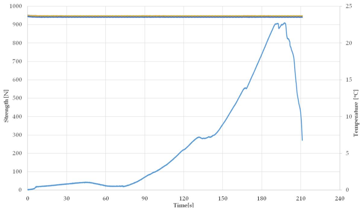
**Figure 10.** Breaking power of the shoe sole at  $20$  °C.
