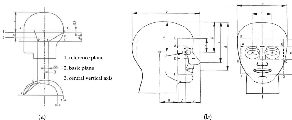
**Figure 2.** Protection zones: (a) 1a—the part above plane AA, 1b—the area between the planes AA and CDEF and 3a—the neck protection zone; (b) 2—comprises at least the eye protection zone defined by EFGH and 3b—comprises at least the CDHG zone.
