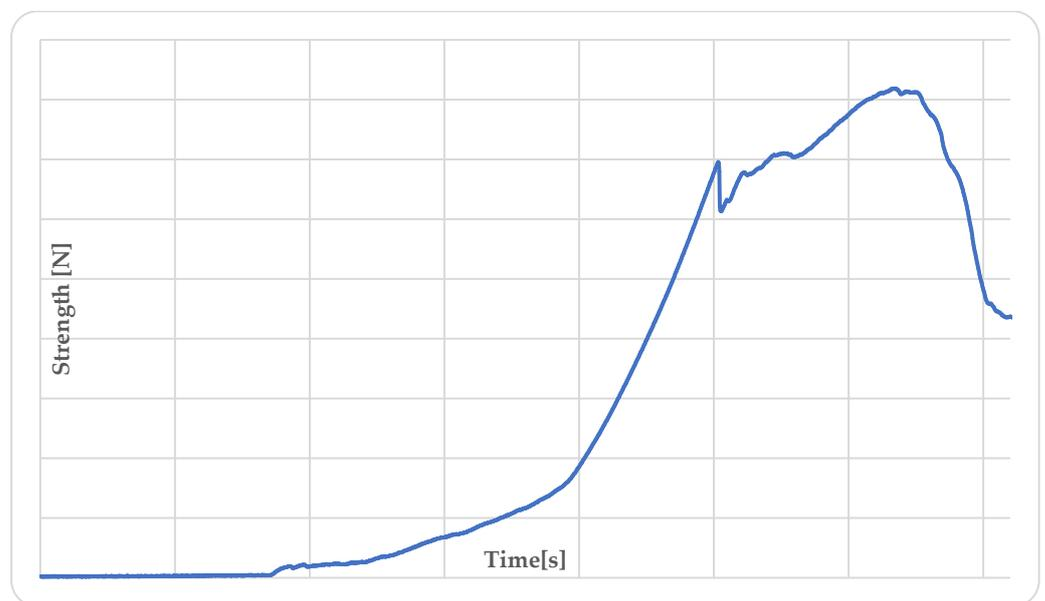
**Figure 13.** Breakthrough force of the shoe sole after cooling the sole to approximately  $-60\text{ }^{\circ}\text{C}$ .
