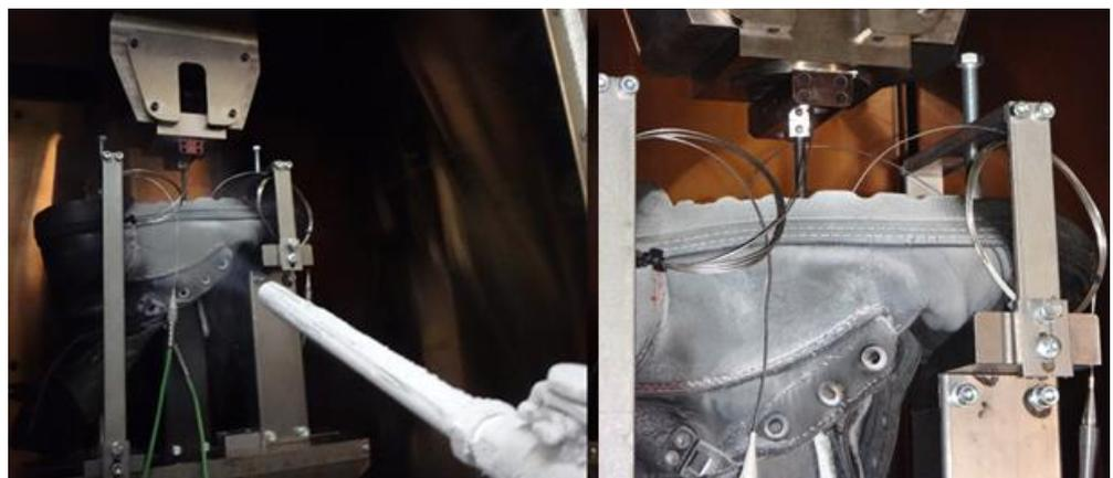
**Figure 11.** Reduction in sole temperatures of special shoes during the puncture test.
