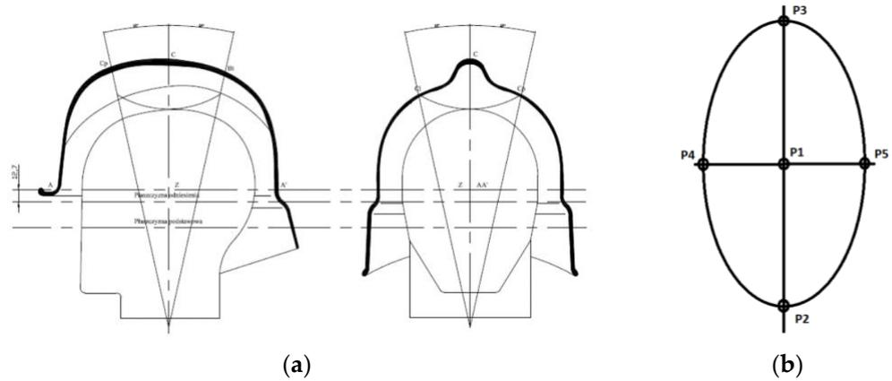
**Figure 4.** Points at which impact was applied: (a) Headform; (b) Measurement points.
