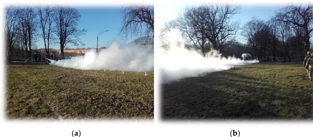
**Figure 1.** LNG expansion during field tests. (a) outflow at a height of 1 meter directed to the ground at an angle of 60 degrees; (b) outflow at a height of 1 meter directed parallel to the ground.
