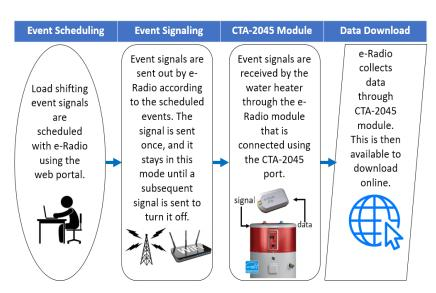
Figure 1. Wireless communication enabled through CTA-2045 module.
