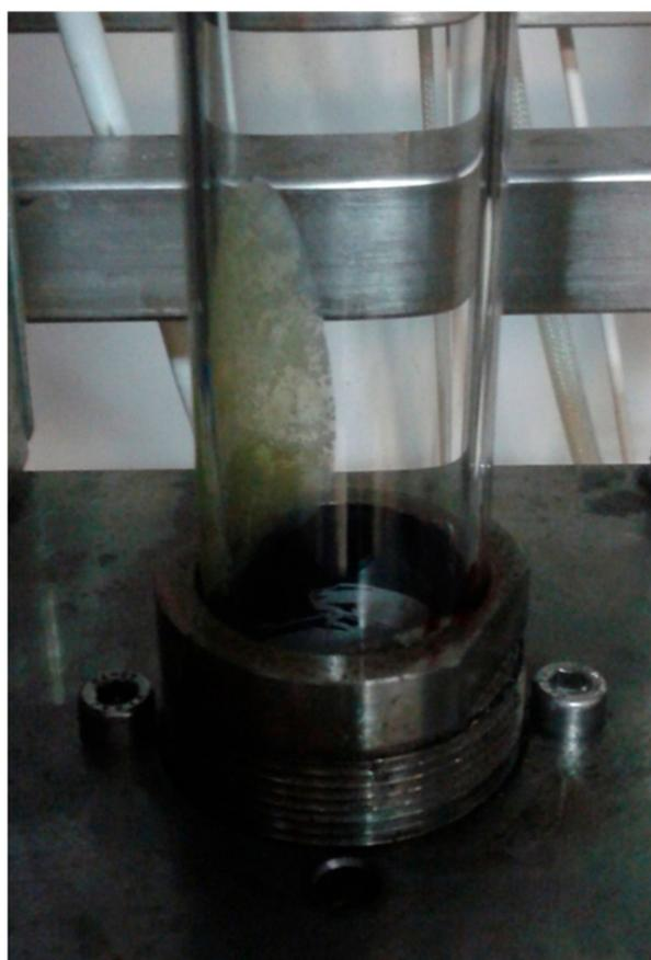
Figure 5. Sulfur deposit on the reactor's wall.
