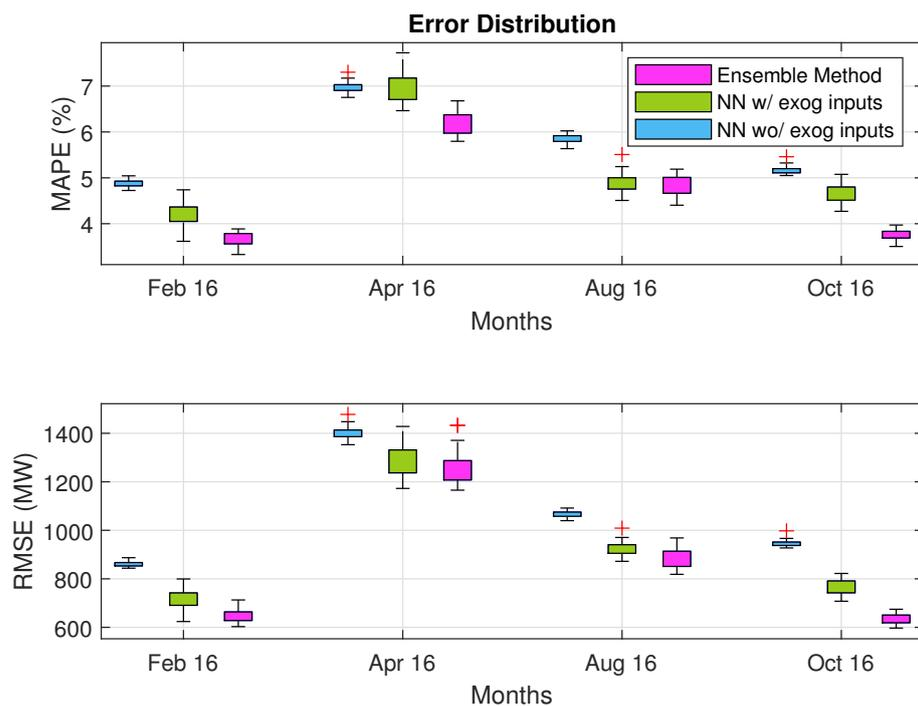
**Figure 6.** Box-plots of the MAPE (%) and RMSE (MW) error distributions (NN without exogenous inputs—blue, NN with exogenous inputs—green and the proposed ensemble methodology—magenta over the course of 50 runs).
