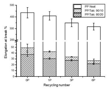
**Figure 10.** Elongation at break of non-recycled and recycled neat PP and PP/talc composites. Reproduced with permission [213].
