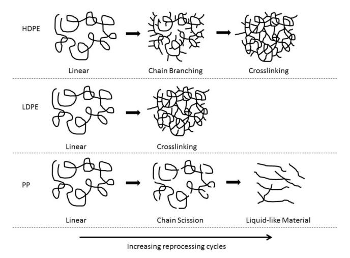
**Figure 6.** Degradation mechanisms of HPDE, LDPE, and PP as the number of reprocessing cycles is increased. Reproduced with permission [154].
