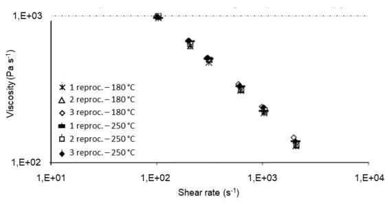
**Figure 7.** Rheological curves of rPP/rHPDE 90/10 wt% under conventional and aggressive temperature conditions. Reproduced with permission [148].
