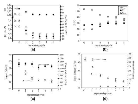
**Figure 16.** Effect of mechanical reprocessing cycles on (a) PDI and viscosity, (b) crystallinity, (c) impact and Young's modulus, and (d) stress and strain at break of PET. Reproduced with permission [315], 2012, Elsevier.
