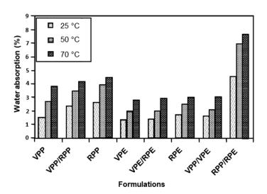
**Figure 11.** Water absorption of virgin and recycled plastic/wood flour composites after 2 h of immersion at three immersion temperatures: 25 °C, 50 °C, and 70 °C. Reproduced with permission [238].
