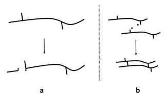
**Figure 5.** Degradation mechanisms: (a) random chain scission and (b) crosslinking. Reproduced with permission [18].
