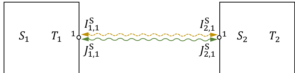
Figure 4. Heat conduction between two reservoirs.
