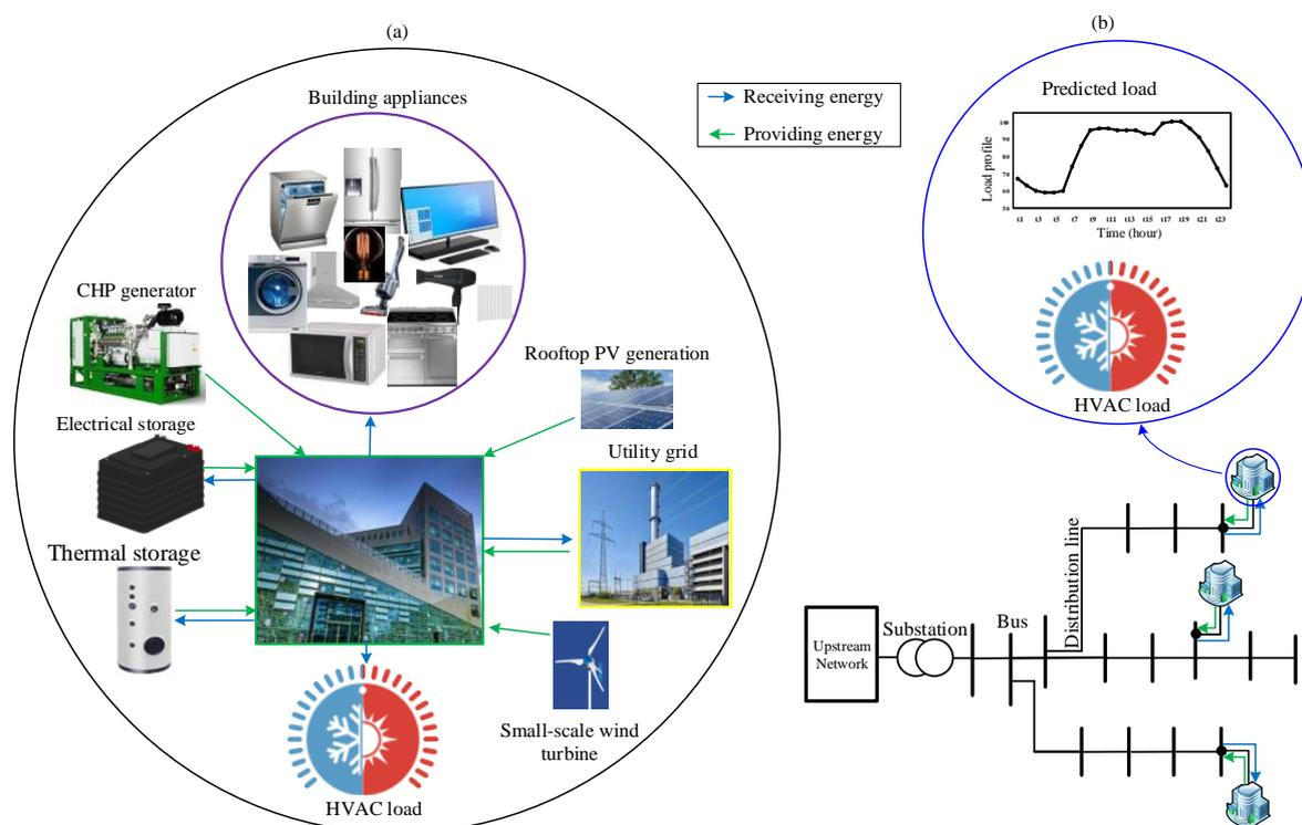
**Figure 3.** Different architectures in integration of ABs into the grid: (a) building-oriented structure, and (b) grid-tied structure.
