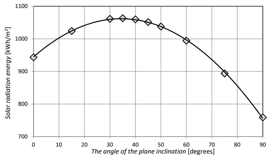
**Figure 12.** The dependence of the total intensity of solar radiation on the slope of the plane directed to the south.
