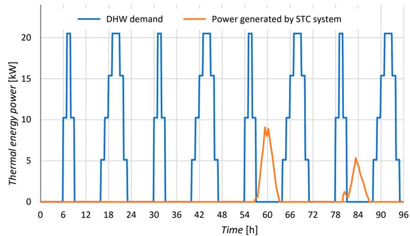
**Figure 9.** Comparison of energy demand for DHW purposes with the amount of energy produced by the STC system from 1 to 4 January.
