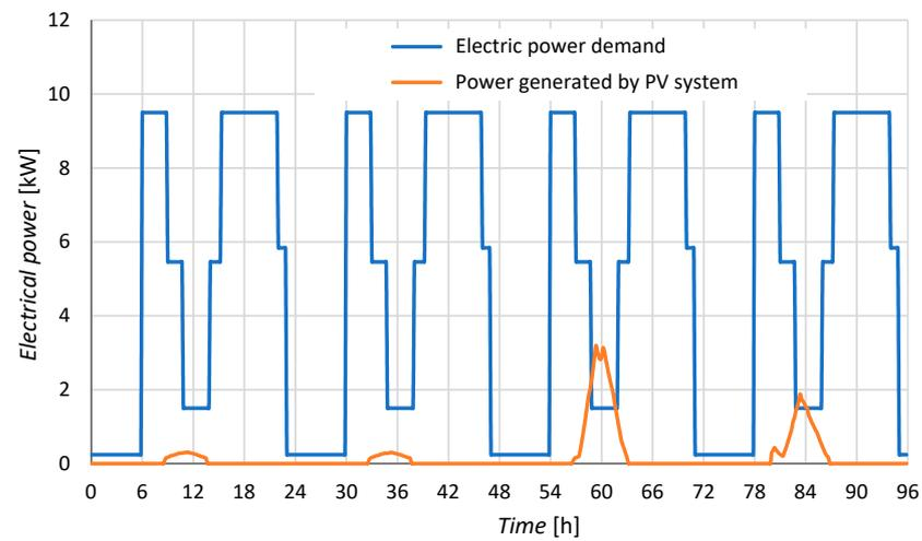
**Figure 8.** Comparison of electricity consumption with the amount of energy produced by the PV system from 1 to 4 January.
