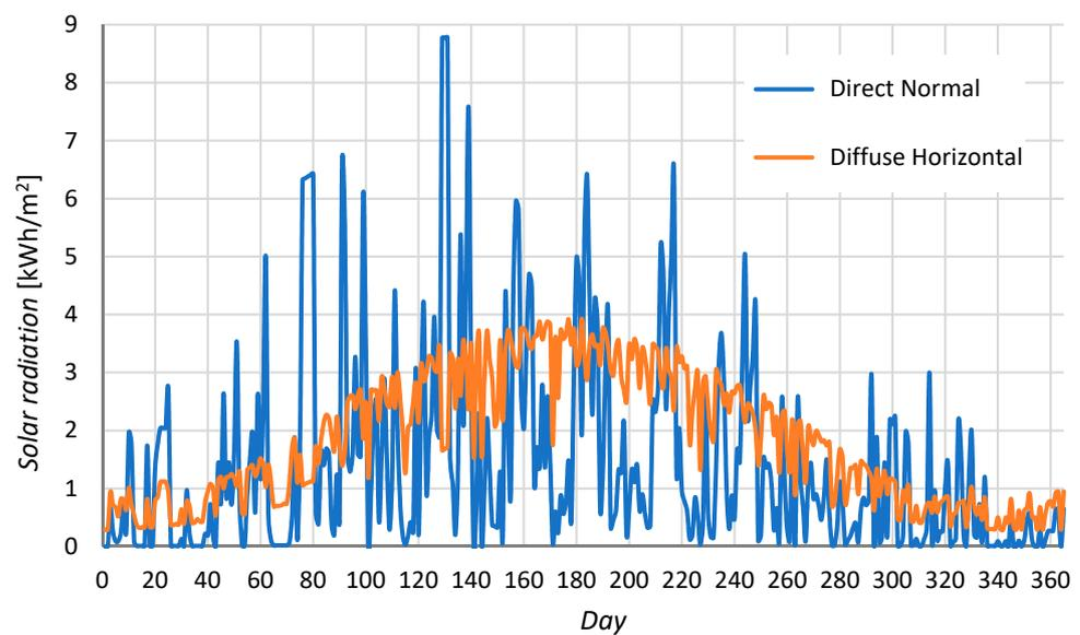
**Figure 6.** Average daily direct and diffuse solar radiation.
