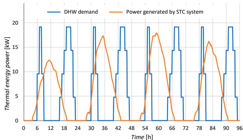
**Figure 11.** Comparison of energy demand for DHW purposes with the amount of energy produced by the STC system from 1 to 4 July.
