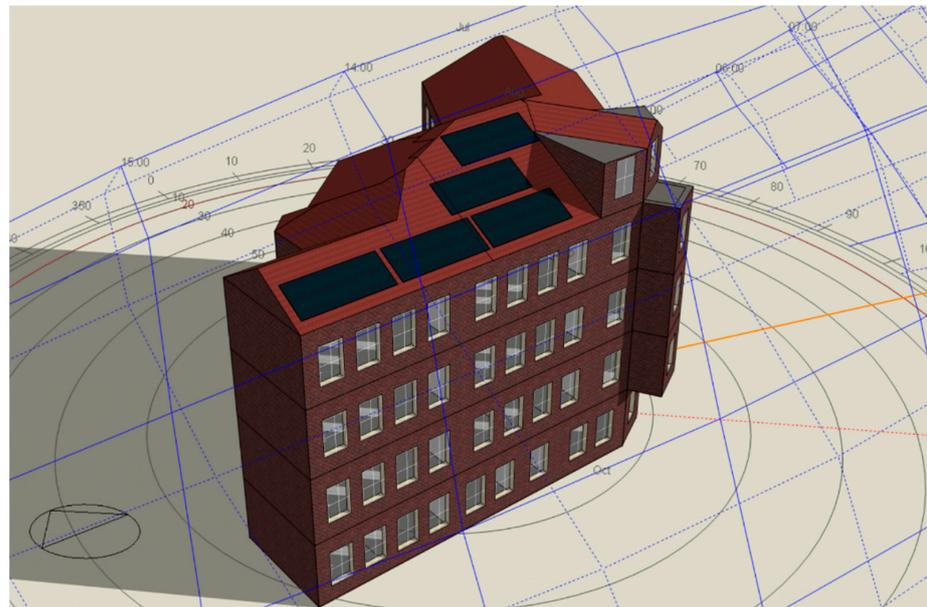
**Figure 1.** Scheme of the arrangement of thermal solar collectors on the roof of the tenement house.
