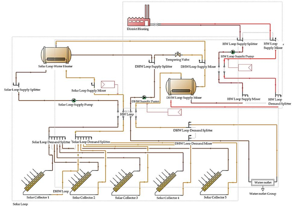
Figure 2. SDHW system developed in DesignBuilder software.
