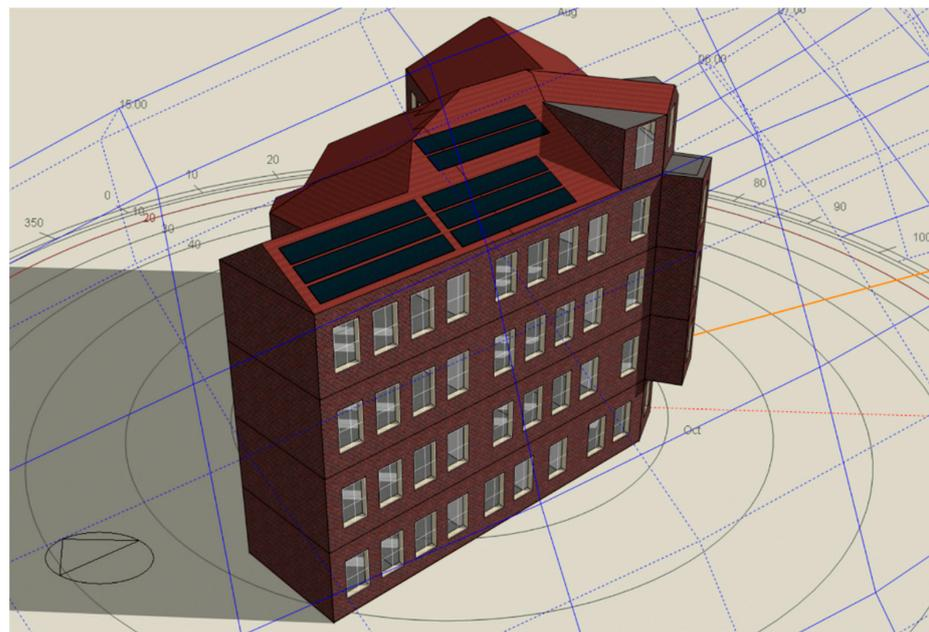
Figure 3. Scheme of the arrangement of photovoltaic panels on the roof of the tenement house.
