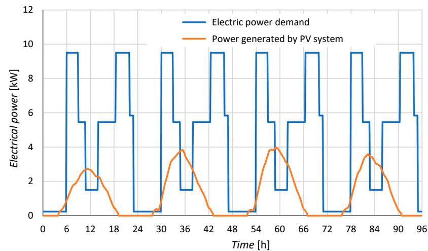
**Figure 10.** Comparison of electricity consumption with the amount of energy produced by the PV system from 1 to 4 July.
