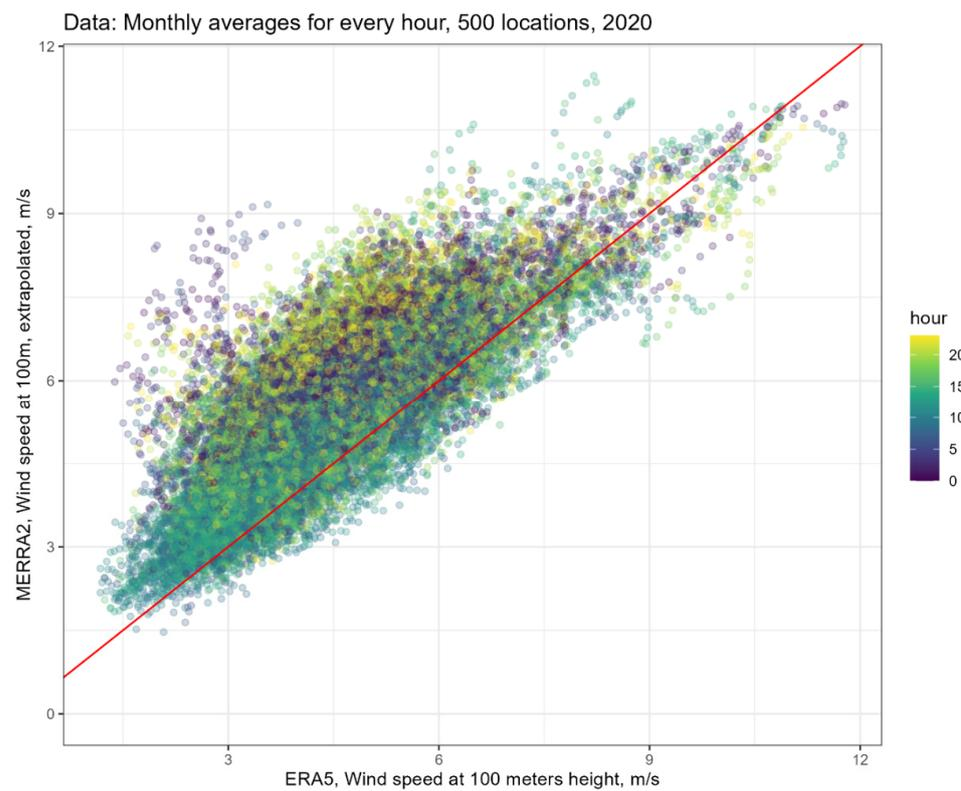
**Figure 7.** Comparison of monthly average wind speed at 100 m height in ERA5 and MERRA-2 (extrapolated from 10 and 50 m heights) datasets.
