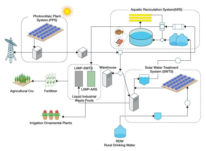
Figure 9. Integrated aquaculture recirculation system plant.
