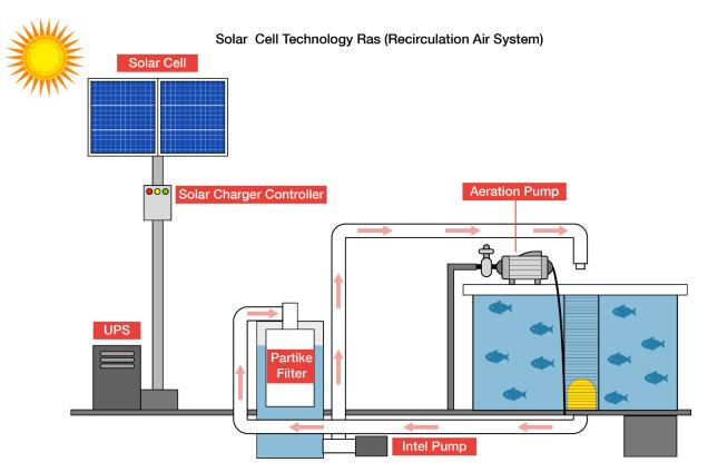
Figure 7. The solar cell recirculated aquaculture system.
