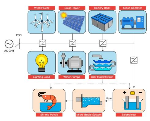
cell, storage systems for oxygen and hydrogen, a micro-bubble generation system, a water treatment system, and an associated load at the shrimp farm (Figure 6).
