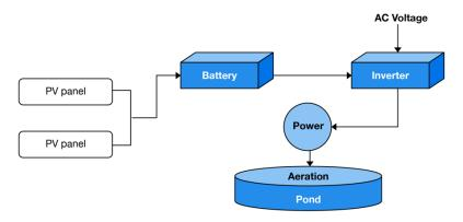
Figure 2. Solar-powered aeration system in an aquaculture pond.
