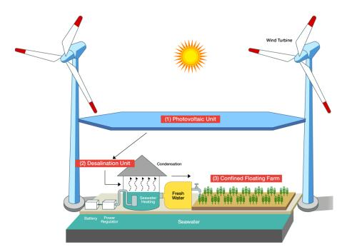
Figure 16. The desalination system for aquaculture/agriculture.
