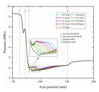
**Figure 14.** Variations of axial static pressure under different  $\theta_{pm}$  ( $P_p$  of 9.3 MPa).
