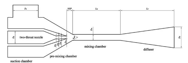
Figure 2. Structural diagram of the two-throat nozzle ejector.
