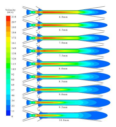
**Figure 9.** Fields of velocity under different  $D_m$  ( $P_p$  of 9.3 MPa).
