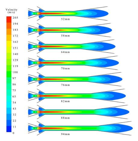
**Figure 12.** Fields of velocity under different  $L_m$  ( $P_p$  of 9.3 MPa).
