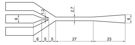
Figure 5. Structural sizes of ejector from the published literature [40].
