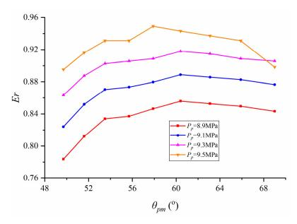
**Figure 13.** Variations of *Er* with different  $\theta_{pm}$  and  $P_p$  ( $D_m$  of 8 mm,  $L_m$  of 64 mm).
