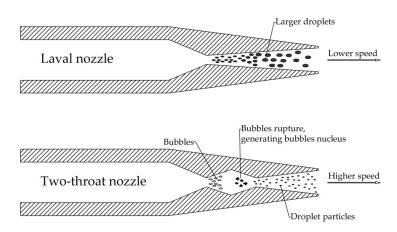
Figure 1. Schematic diagram of a two-throat nozzle and a Laval nozzle.
