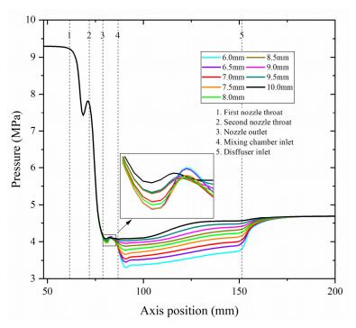
**Figure 8.** Variations of axial static pressures under different  $D_m$  ( $P_p$  of 9.3 MPa).
