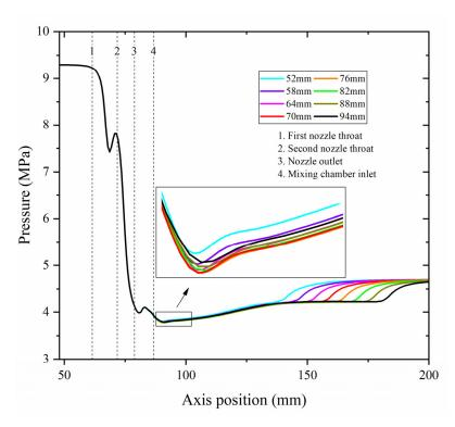
**Figure 11.** Variations of axial static pressures under different  $L_m$  ( $P_p$  of 9.3 MPa).
