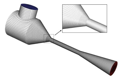
Figure 3. Grid of the two-throat nozzle ejector 3D model.
