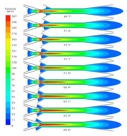
**Figure 15.** Fields of velocity under different  $\theta_{pm}$  ( $P_p$  of 9.3 MPa).
