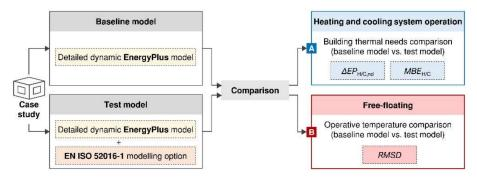
**Figure 1.** Methodology framework applicable for the energy need (**A**) and the indoor temperature (**B**) evaluations.
