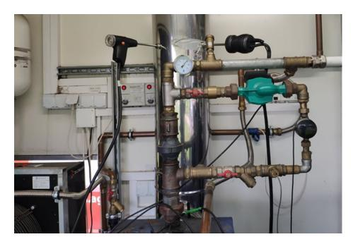
Figure 5. Chimney with flue gas probes installed. Testo 350 probe on the left, FSM probe on the right.
