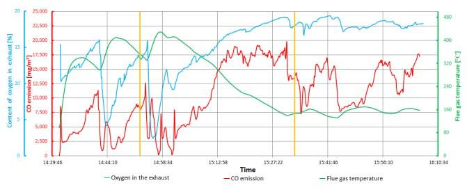
**Figure 7.** The oxygen in the exhaust and CO emission relative to 10% oxygen content in flue gas, birch wood billet. The yellow lines indicate the period of dust measurement.
