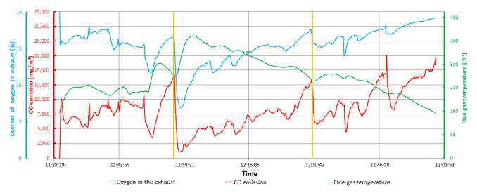
**Figure 11.** The oxygen in the exhaust and CO emission relative to 10% oxygen content in flue gas, beech wood billet. The yellow lines indicate the period of dust measurement.
