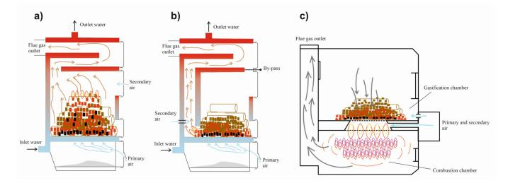
**Figure 1.** Boiler designs: (**a**) boilers with updraft combustion, reproduced from the work of [30]; (**b**) boilers with downdraft combustion, reproduced from the work of [30]; (**c**) gasification boilers, reproduced from the work of [31].
