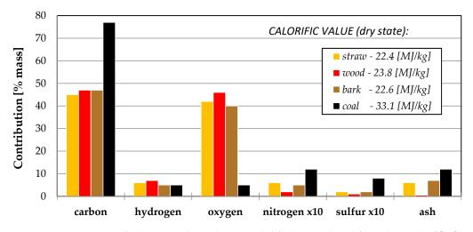
Figure 2. Proportion of substances depending on solid fuel, reproduced from the work of [32].
