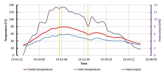
**Figure 6.** The operation parameters of the system and heat output of the boiler achieved during the combustion of birch wood billet. The yellow lines indicate the dust measurement period.
