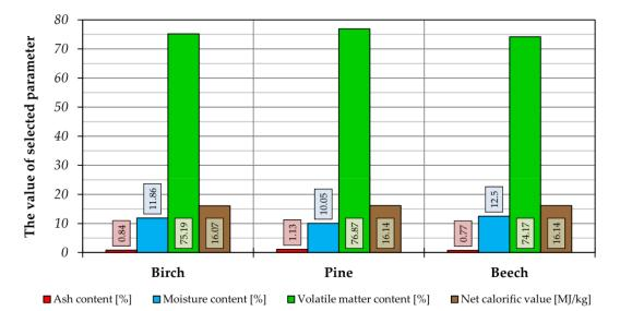
Figure 12. Summary of average physicochemical parameters of the three types of wood billets tested.
