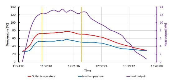
**Figure 10.** The operation parameters of the system and heat output of the boiler achieved during the combustion of beech wood billet. The yellow lines indicate the dust measurement period.
