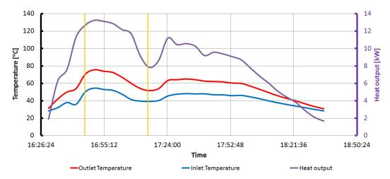
**Figure 8.** The operation parameters of the system and heat output of the boiler achieved during the combustion of pine wood billet. The yellow lines indicate the dust measurement period.
