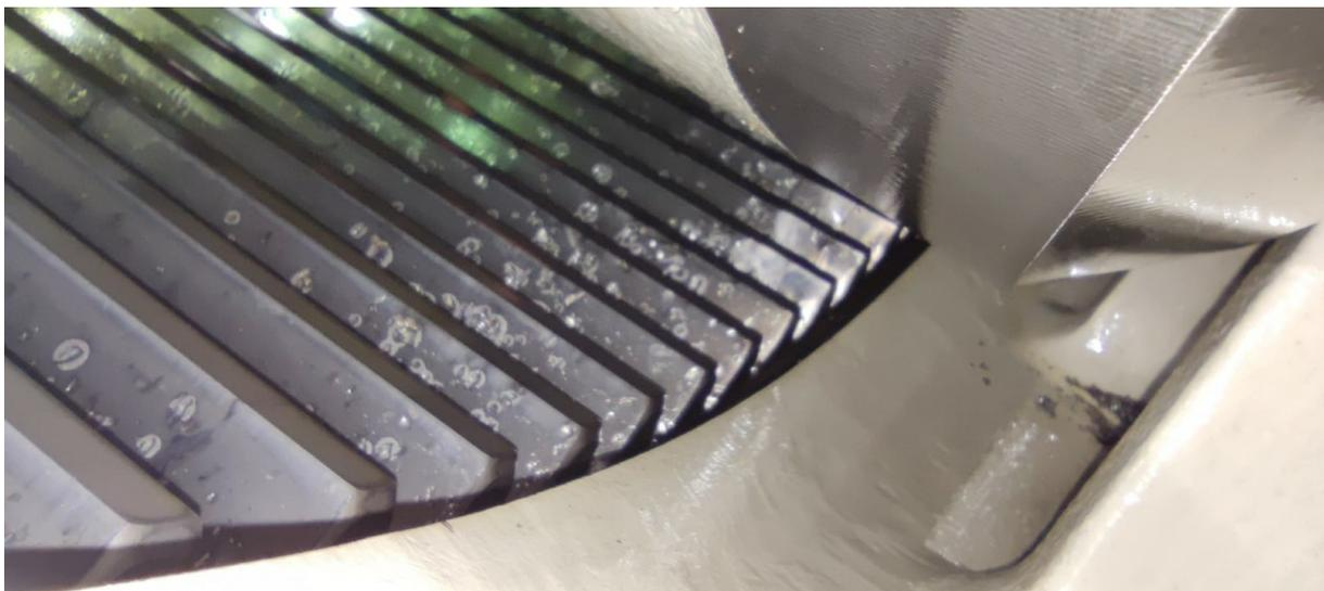
**Figure 6.** The effect of planetary gear teeth wear in wind turbines in the form of spots caused by gases released inside the nacelle.
