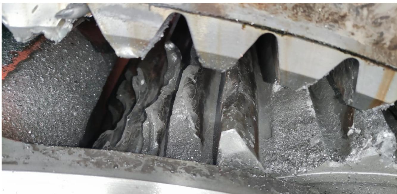
**Figure 11.** Total break-off of toothed wheel fragments in the wind turbine planetary gear.
