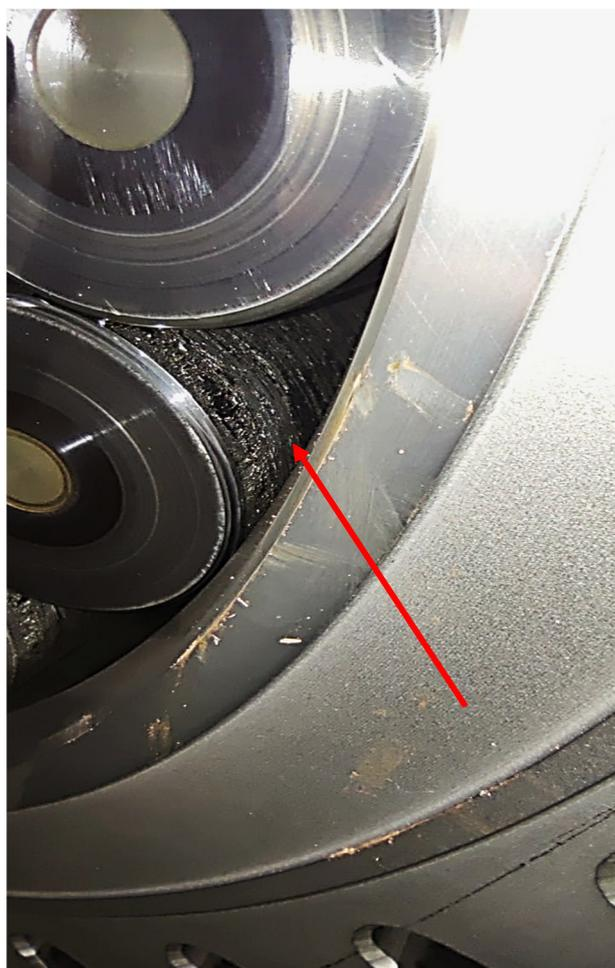
**Figure 12.** Bearing elements with visible heat-adhesion damage (arrow).
