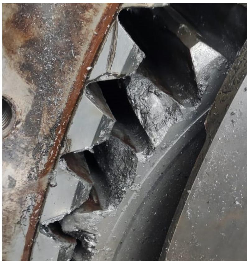
**Figure 10.** Broken off fragment of a planet wheel tooth in the planetary gear.
