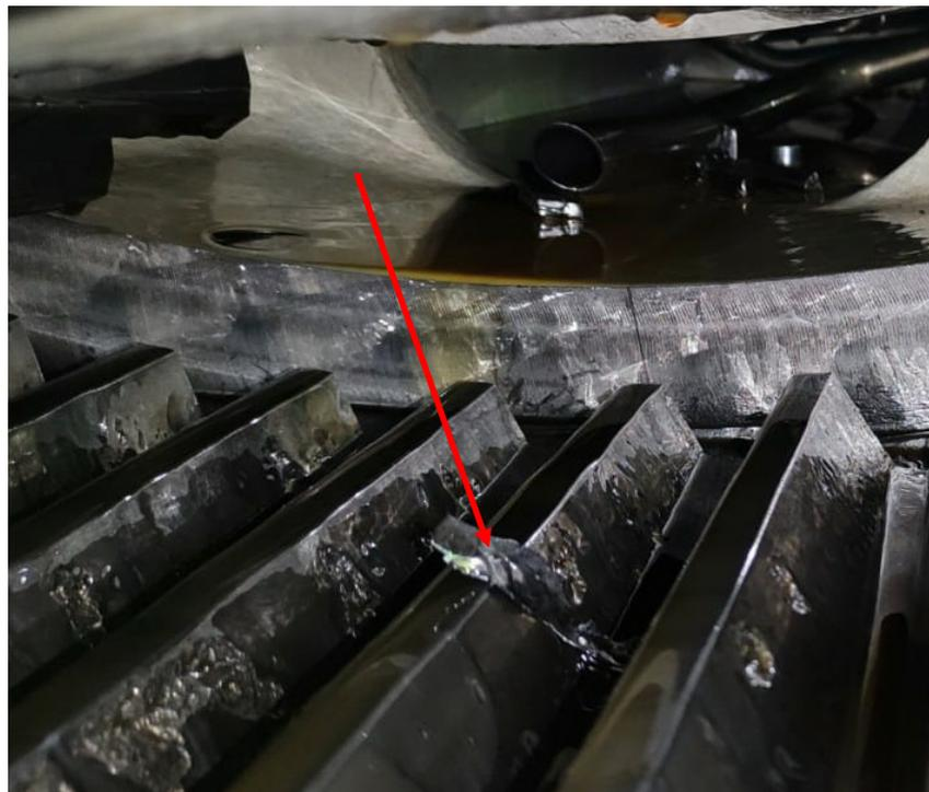
**Figure 9.** Breaking off material particles from the surface layer (arrow).
