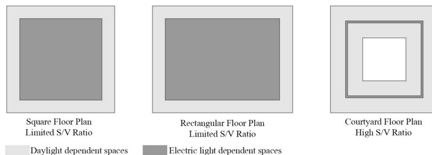
**Figure 9.** Increasing the S/V ratio provides better daylight inside spaces.
