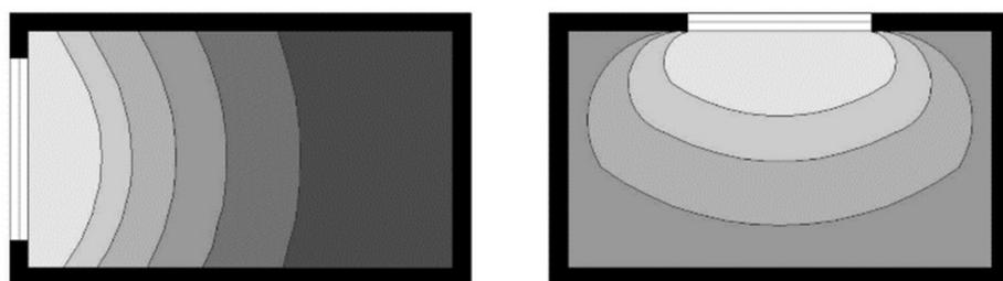
**Figure 3.** Luminous uniformity in rectangular space in relation to window placement within different façades.
