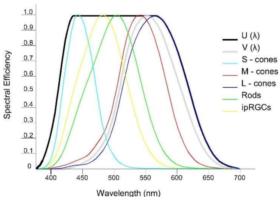
**Figure 11.** The spectral efficiency function of  $U(\lambda)$ ,  $V(\lambda)$ , and the known photoreceptors (adapted from [101]).
