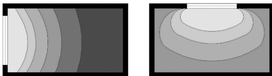
**Figure 3.** Luminous uniformity in rectangular space in relation to window placement within different facades.
