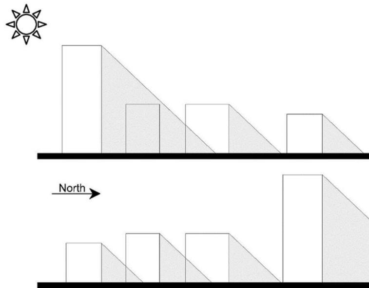
**Figure 2.** In the Northern hemisphere, placing tall buildings on the south of urban fabric prevents daylight access to low buildings.
