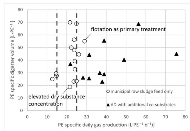
**Figure 3.** PE-specific digester volume ( $L \cdot PE^{-1}$ ) and PE-specific daily gas production ( $L \cdot PE^{-1} \cdot d^{-1}$ ) for 28 Austrian municipal digesters: ADs including co-substrate dosing are marked with triangles; the expected range for the specific gas production from the literature ( $15\text{--}25 L \cdot PE^{-1} \cdot d^{-1}$ ) is marked with dashed lines.
