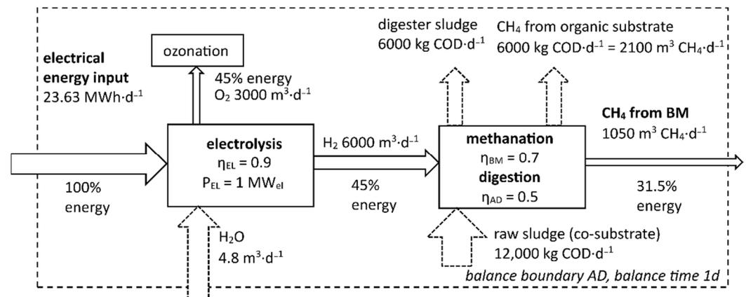
**Figure 4.** Energy and mass flow chart for in situ methanation in municipal digesters: values calculated for a 100,000 PE model WWTP with AD.
