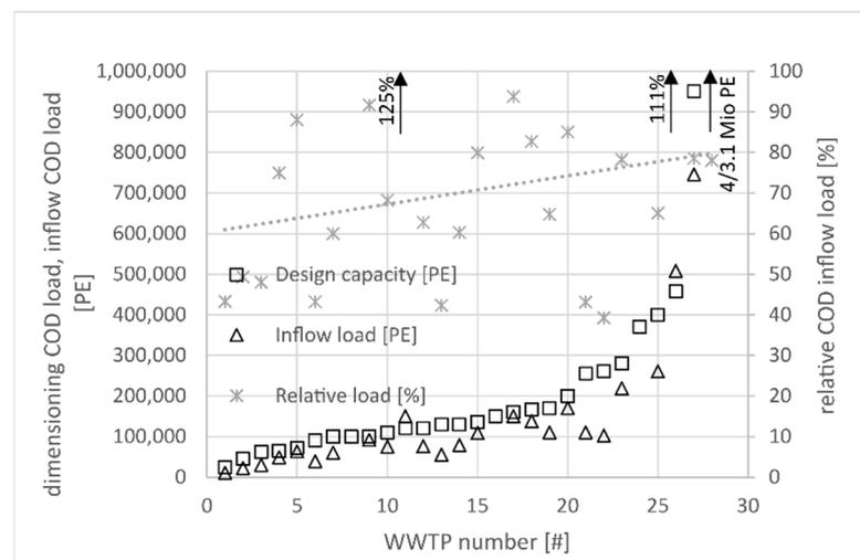
**Figure 2.** Design capacity  $PE_{COD}$  (squares), inflow load  $PE_{COD}$  (triangles) and relative COD load (stars) of 28 Austrian WWTPs.
