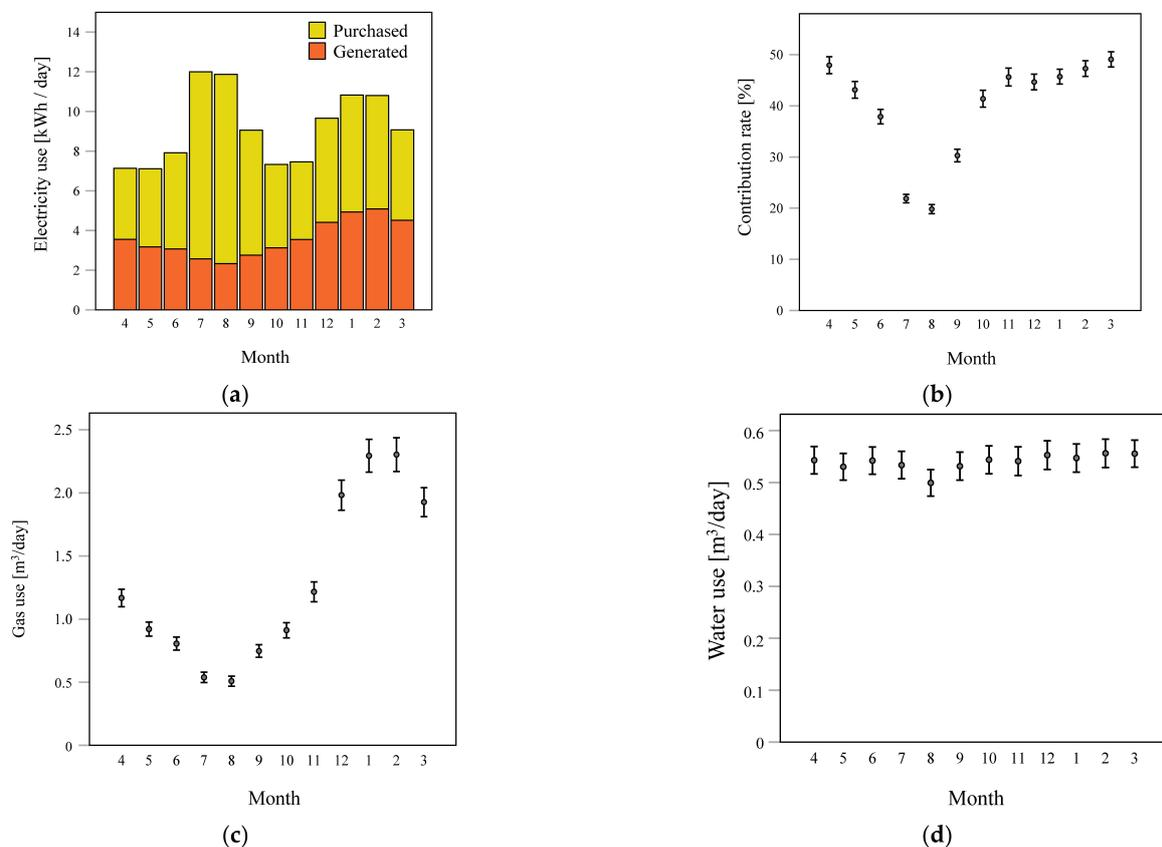
**Figure 8.** Monthly variation (n = 304): (a) electricity use; (b) contribution rate; (c) gas use (except for CGS); (d) water use.
