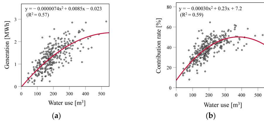
**Figure 6.** Relationship between the annual water use and the energy-saving effects of CGS in each household (n = 304): (a) generation; (b) contribution rate.
