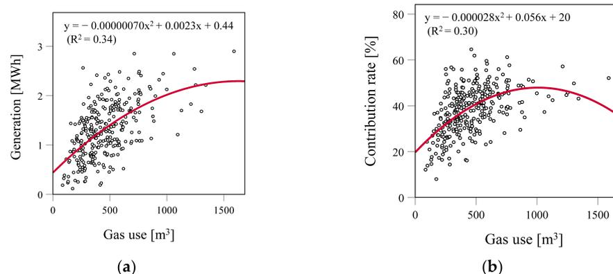
**Figure 5.** Relationship between the annual gas use (except for CGS) and the energy-saving effects of CGS in each household ( $n = 304$ ): (a) generation; (b) contribution rate.
