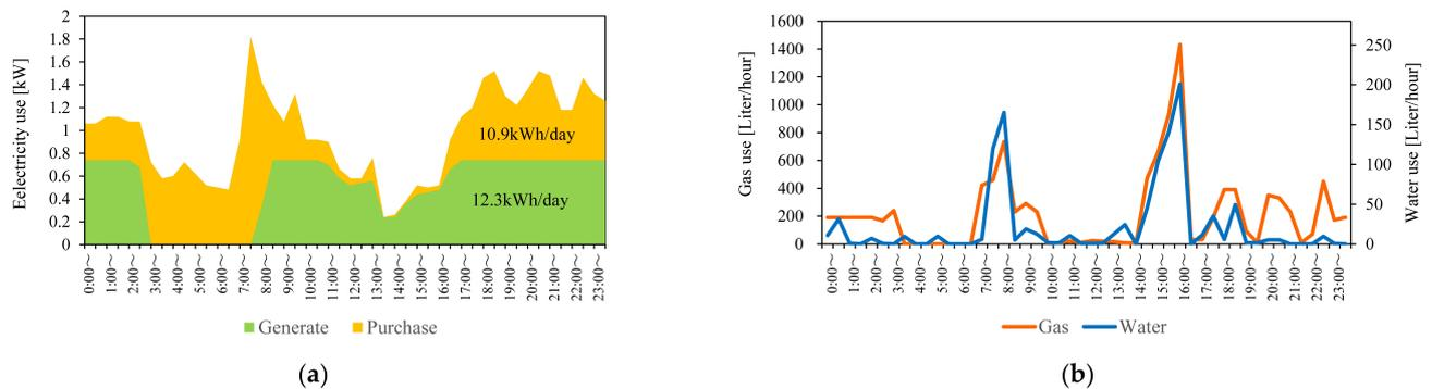
**Figure 3.** Variation of daily energy use (example data of a flat on 1 February): (a) electricity generated by CGS and purchased; (b) gas use (except for CGS) and water use.
