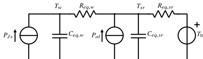
Figure 3. Second-order thermal model including the thermal parameter involved with the thermal conduction only.
