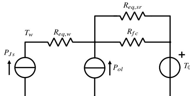
Figure 4. Steady-state thermal network in load condition.
