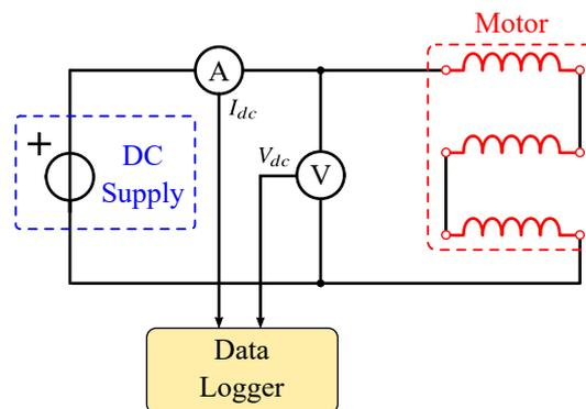
Figure 2. Experimental configuration of the dc test.
