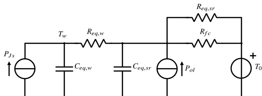
Figure 1. Second-order thermal model proposed in [13].
