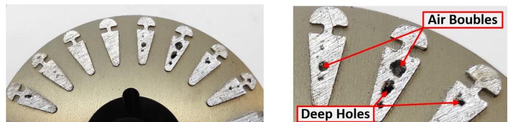
Figure 29. Cut in 1/3 of the length of the sample R3.
