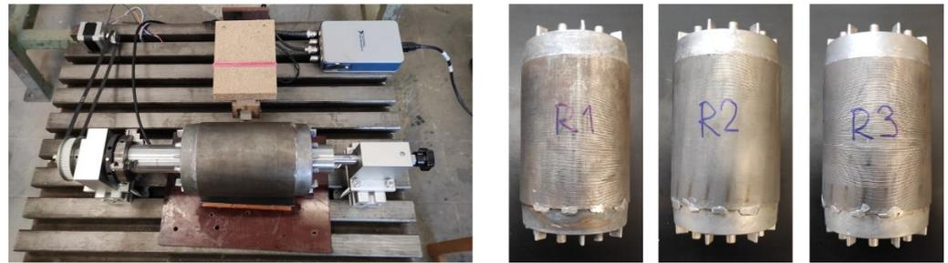
Figure 24. Measurement system for real rotor testing.
