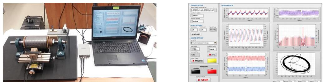
**Figure 16.** Completed experimental setup with visualization panel in LabView.
