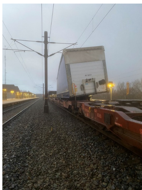
Figure 1. In 2021 during the passage of a freight train over the bridge, the semi-trailer was forced out of its attachment (strong wind and empty trailer), source: utk.gov.pl [8].
