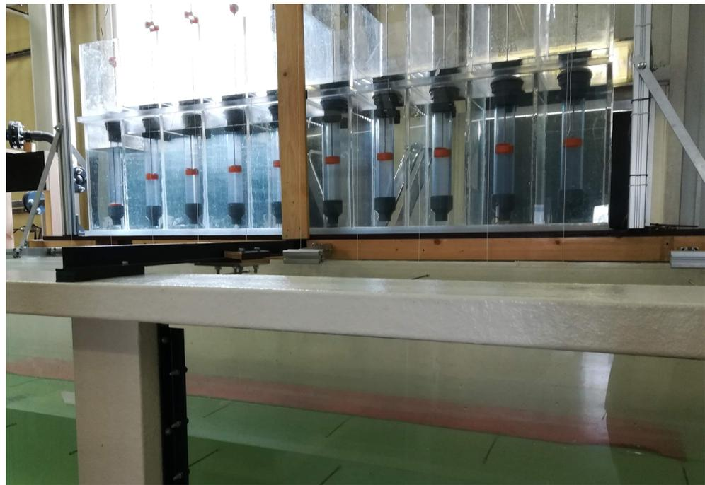
**Figure 19.** Laboratory demonstration of the flexible floater (red silicone sheet inside the tank) connected to the MP<sup>2</sup>PTO system at the University of Groningen.
