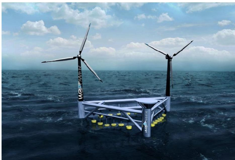
**Figure 8.** Artist’s sketch of the W2Power hybrid wind–wave system. Image taken from Ref. [44] “McTiernan, K.L.; Sharman, K.T. Review of Hybrid Offshore Wind and Wave Energy Systems. *J. Phys. Conf. Ser.* **2020**, *1452*, 012016.” Copyright 2020 Author(s), licensed under a Creative Commons Attribution (CC BY 3.0) license.
