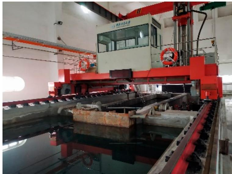
**Figure 10.** Towing system for the Unmanned Underwater Delivery Technology Laboratory.
