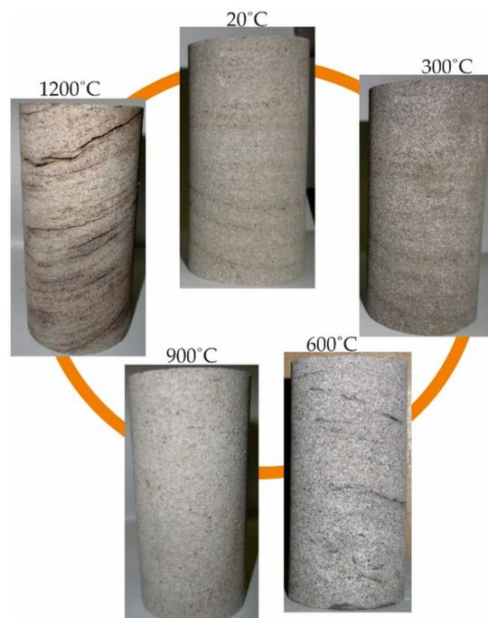
Figure 4. Sandstone heated at high temperatures.
