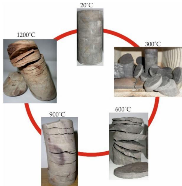
Figure 3. Claystone heated at high temperatures.
