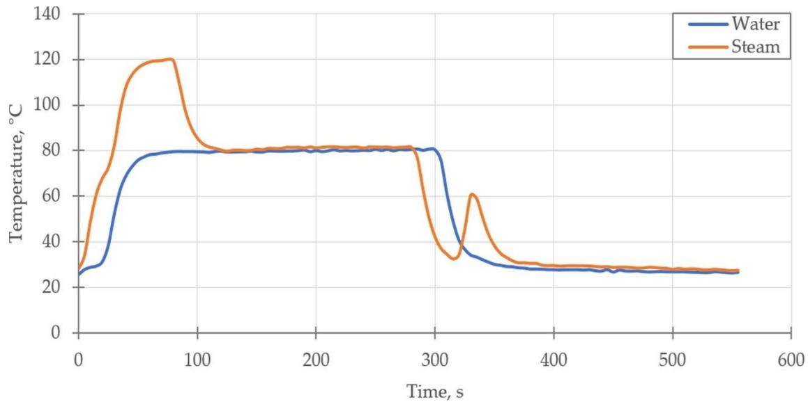
**Figure 3.** Temperature of the medium inlet (T5) to the adsorption chiller bed during desorption.
