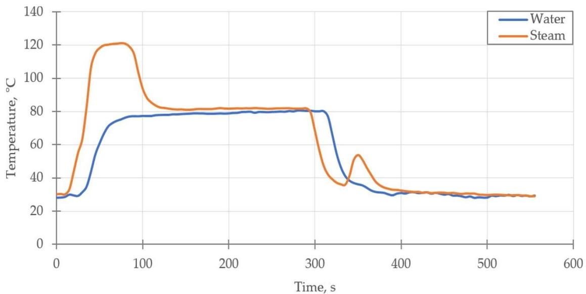
**Figure 4.** Temperature of the medium outlet (T7) from the adsorption chiller bed during desorption.
