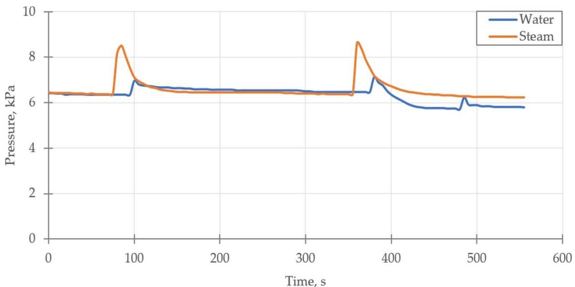
**Figure 9.** Pressure inside the condenser (P4).
