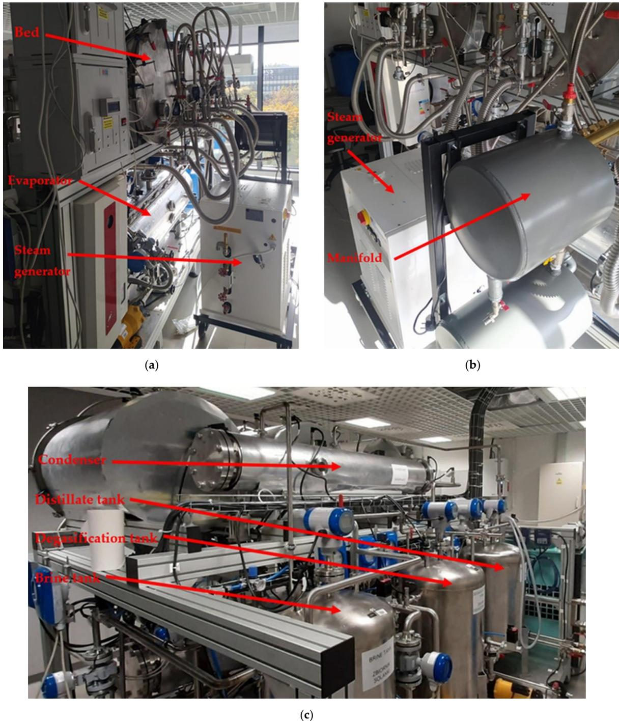
**Figure 2.** Pictures of the test stand: (a) front view on the beds, evaporator and steam generator; (b) front view on the steam generator and manifold; (c) back view on the condenser, distillate tank, degasification tank and brine tank.
