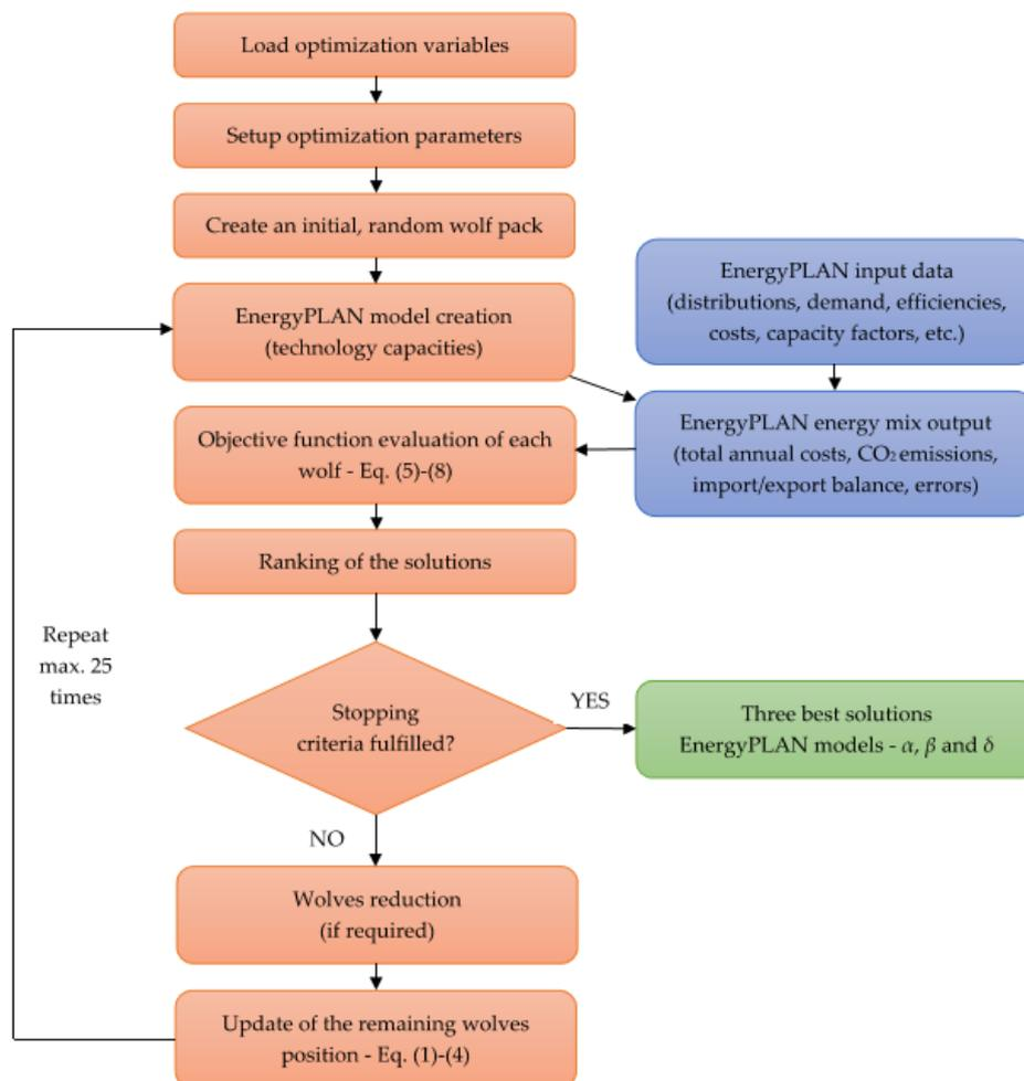
**Figure 5.** Diagram of the optimization process and the interaction between MATLAB (orange box) and EnergyPLAN (blue box).
