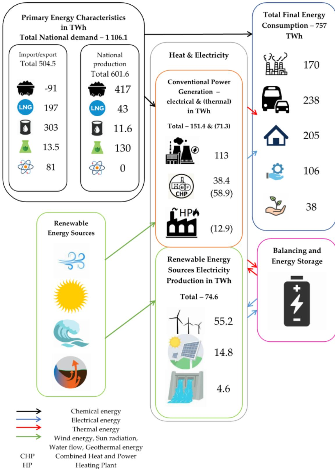
Figure 3. Flowchart of the Polish energy system.
