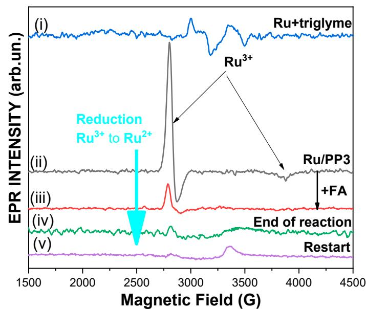
**Figure S4.** EPR spectra of the catalytic system. (i) only the Ru-precursor in triglyme (ii) [Ru/PP3] catalyst in triglyme after 10 min (iii) catalytic reaction ([Ru/PP3]/FA/KOH in triglyme:water solution) during evolution (iv) after the end of the catalytic reaction and (v) restart of catalytic reaction by adding 1 ml of FA on the next day.
