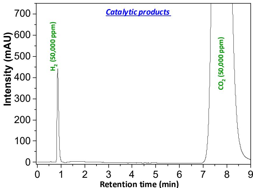
**Figure S1.** Representative GC-TCD chromatogram for the catalytic gas products, detected by a Shimadzu GC-2014 GC-TCD with a Carboxen-1000 column.
