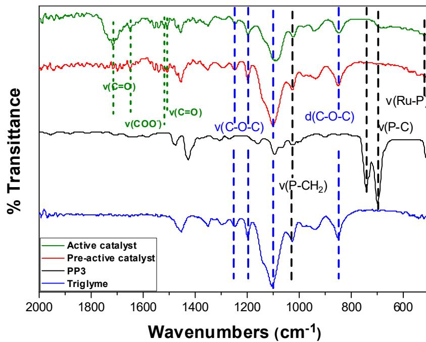
**Figure S3.** ATR spectrum for all components in the catalytic system.
