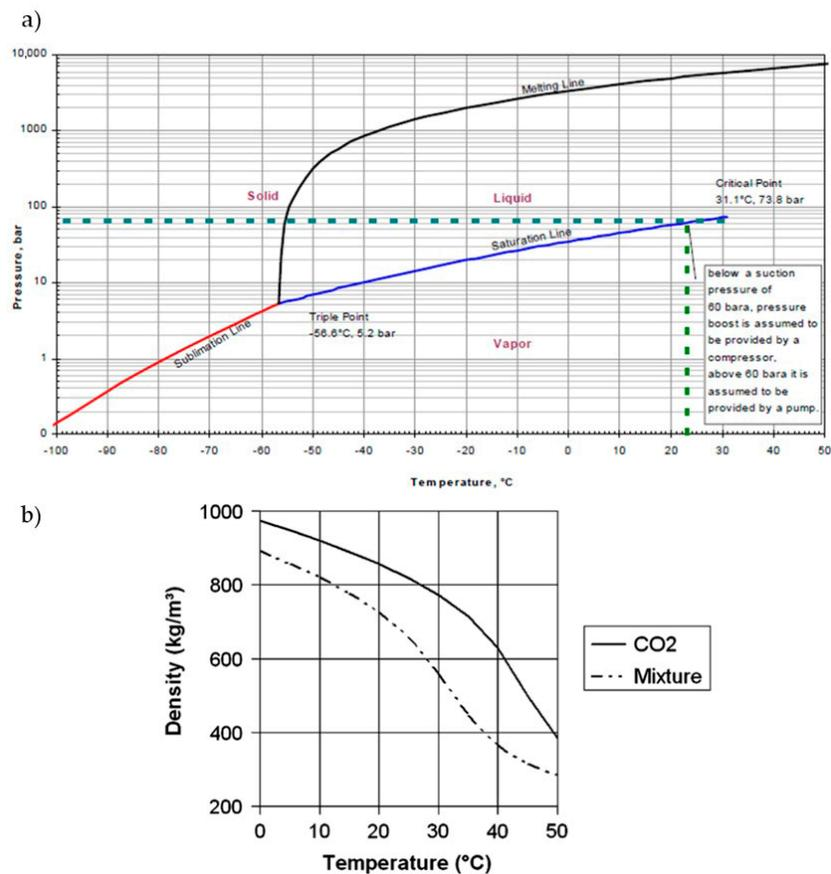
**Figure 9.** (a) CO<sub>2</sub> phase diagram; (b) difference in density of pure CO<sub>2</sub> and CO<sub>2</sub> rich mixture [95% CO<sub>2</sub>/3% N<sub>2</sub>/2% O<sub>2</sub>] at 100 bar. International Energy Agency (IEA) [Woodhill] (2002) Pipeline transmission of CO<sub>2</sub> and energy transmission study-report. All rights reserved [39].
