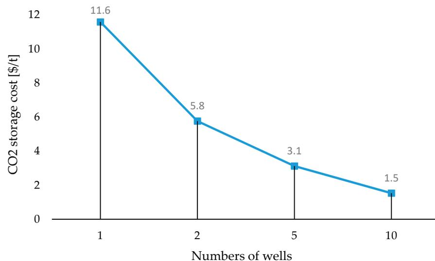
**Figure 14.** CO<sub>2</sub> storage cost at different numbers of wells when a combined method that includes CO<sub>2</sub> replacement and depressurisation of the NGH reservoir is applied to produce methane.
