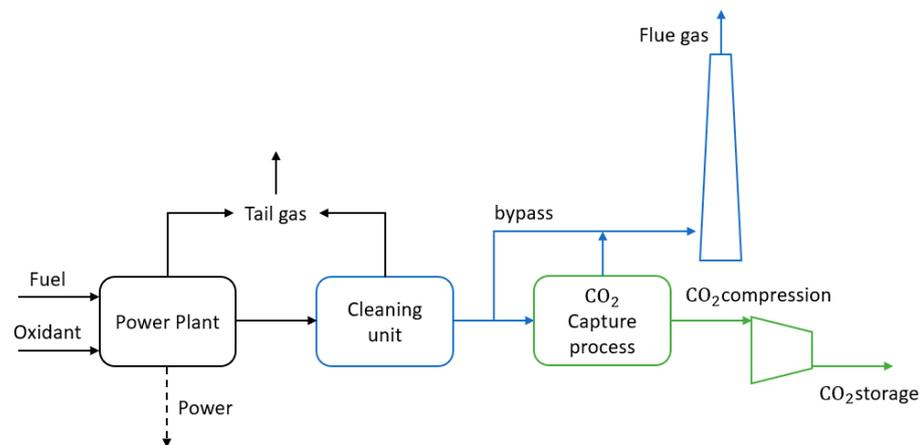
**Figure 5.** Block flow diagram of power plant with post-combustion CO<sub>2</sub> capture technology.
