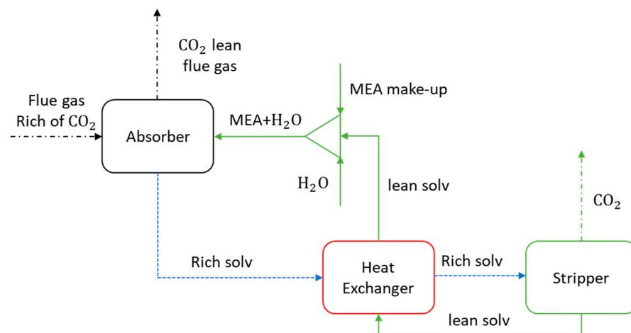
**Figure 6.** Scheme of post-combustion CO<sub>2</sub> capture with a chemical absorption process using aqueous monoethanolamine (MEA) solution.
