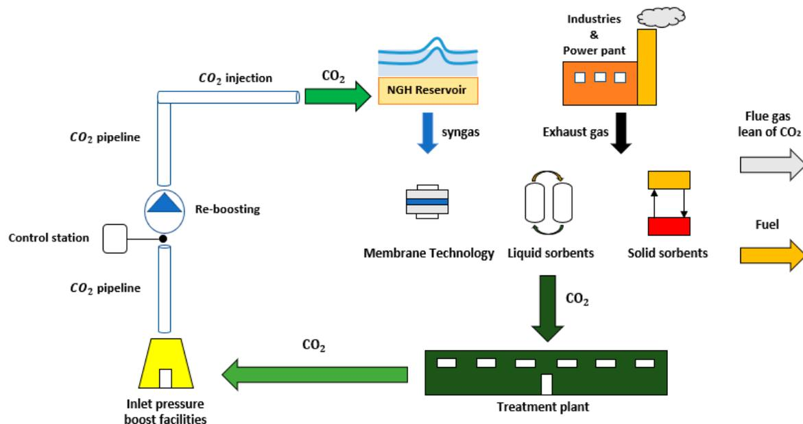
**Figure 18.** Final CCS chain. The flue gas from industries and power plants is treated into the separation unit. The CO<sub>2</sub> captured is transported via pipeline to the NGH reservoir. The injection of CO<sub>2</sub> causes a syngas production. The syngas was purified through membrane technology, and the permeant gas-rich of CO<sub>2</sub> will be injected another time in NGH reservoir. The fuel product rich of methane is in this way a neutral carbon fuel.
