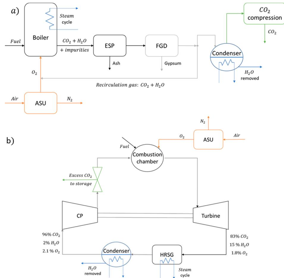
**Figure 3.** (a) Oxyfuel combustion in the Circulating Fluidised Bed (CFB) reactor with CO<sub>2</sub> recirculation coupled with Rankine cycle (secondary cycle); (b) gas turbine cycle with CO<sub>2</sub> recirculation (direct cycle). In both plants, the storage receives near pure excess of CO<sub>2</sub> [24].
