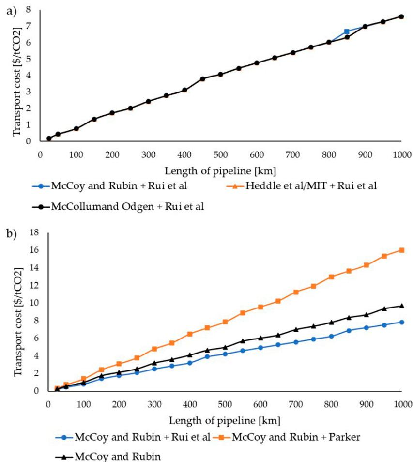
**Figure 10.** CO<sub>2</sub> transport cost computed with 2013 in dollars. (a) To obtain this graph, three different methods are used to calculate the inner diameter while the same method (Rui et al.) is used for the economic analysis. (b) In this graph, we used the same method (McCoy and Rubin) to compute the inner diameter, while various ways are used to carry out the economic analysis.
