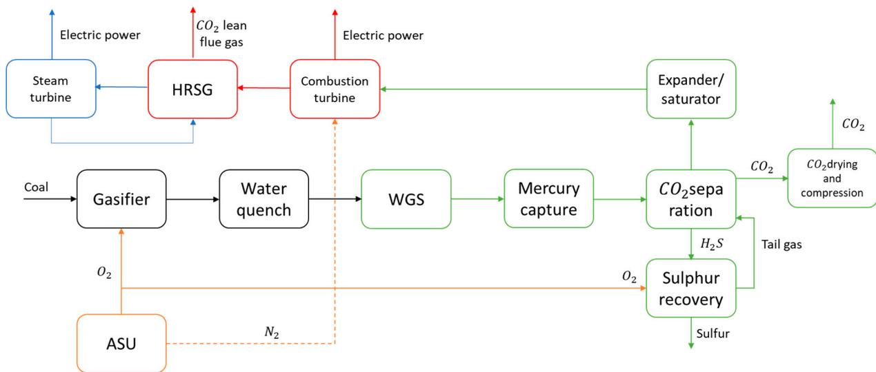
Figure 4. IGCC block flow diagram with CO<sub>2</sub> capture.
