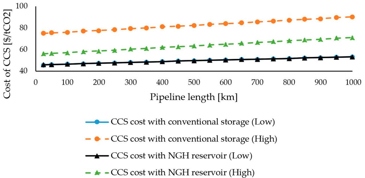
**Figure 16.** Cost of CCS at a different distance between source and storage. The continuous line represents the lower cost of CCS, while dashed lines are the higher value of CCS. The triangles indicate the CCS cost chain when methane is produced via depressurization and the CO<sub>2</sub> replacement, while the circles indicate the CCS cost chain with conventional storage sites described in Table 8.
