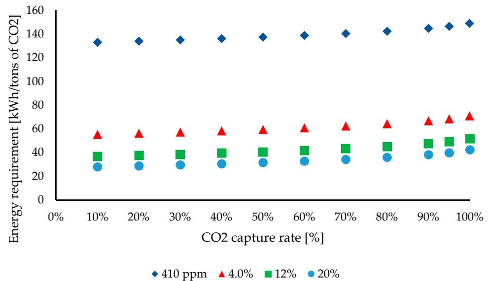
**Figure 2.** Minimum energy requirement for CO<sub>2</sub> capture depending on the capture rate and inlet concentration of CO<sub>2</sub> at 50 °C.  $W = -RT \left\{ \ln \left[ \frac{(1-f)x}{1-fx} \right] + \frac{\ln(1-fx)}{fx} - \frac{\ln(1-f)}{f} \right\}$  [19].
