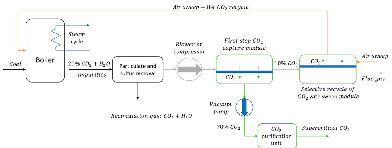
**Figure 8.** Simplified diagram of the Membrane and Technology Research Institute (MTR) selective recycle CO<sub>2</sub> capture process at a coal-fired power plant using Polaris™ membrane in separation modules [22].
