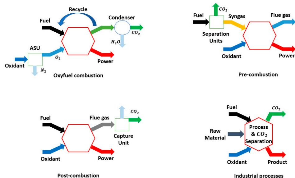
**Figure 1.** Schematic diagrams of carbon capture processes showing oxyfuel combustion, pre-combustion, and post-combustion applied to the energy sector, while the last diagram illustrates a general  $\text{CO}_2$  separation process for a net-zero industry.
