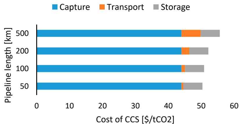
**Figure 17.** Total cost of CCS chain for several pipeline length, subdivided into the three components: capture, transportation, and storage in NGH. For the transportation cost was used a mean value while for the storage cost in NGH reservoir was assumed two wells.
