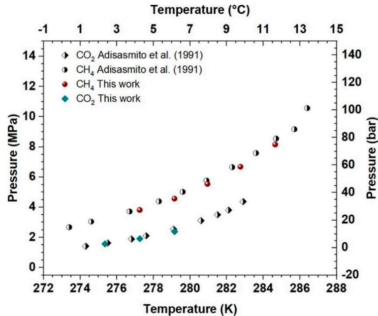
**Figure 11.** Phase diagram (equilibrium temperature as a function of pressure) for pure CO<sub>2</sub> and pure CH<sub>4</sub> gas hydrates [50]. Reprinted from Applied Energy, Vol 280/edition number 115,843, Quang-DuLe et al. Influence of the initial CH<sub>4</sub>-hydrate system properties on CO<sub>2</sub> capture kinetics, Copyright (2020), with permission from Elsevier.
