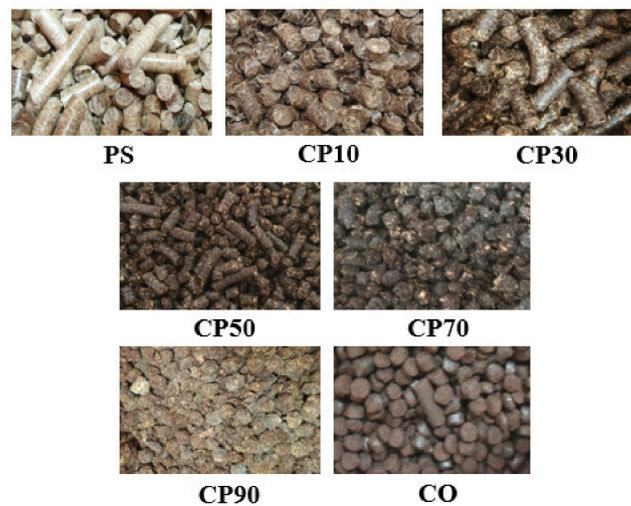
**Figure 3.** Pellets produced using various blending ratios of SCG and pine sawdust (PS).
