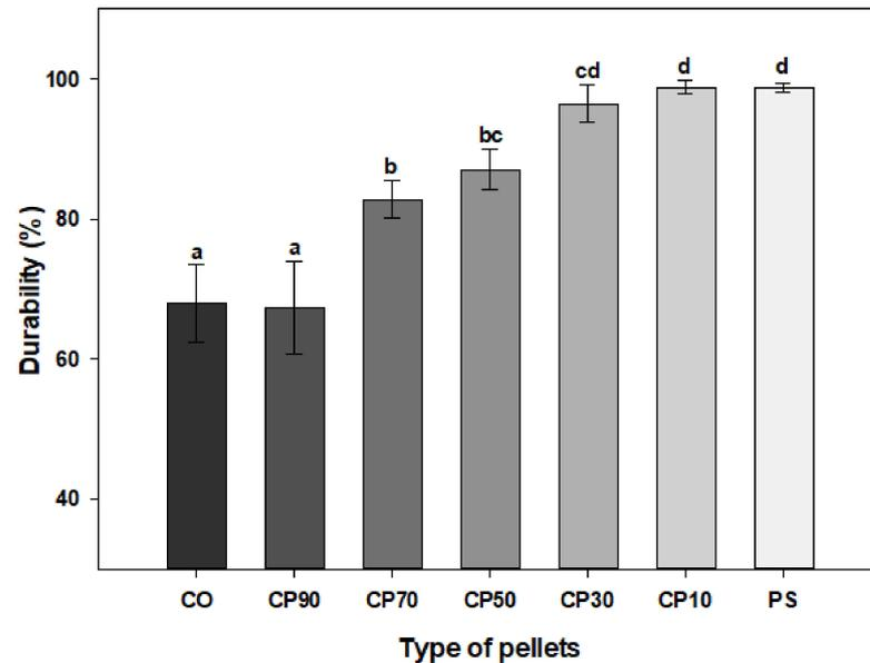
**Figure 6.** Pellet durability according to SCG blending ratio. Each point is the mean of three repeated measurements and is the mean  $\pm$  standard deviation. The means with different letters (a–d) above the bars indicate significant differences based on Tukey’s HSD test ( $p < 0.05$ ).
