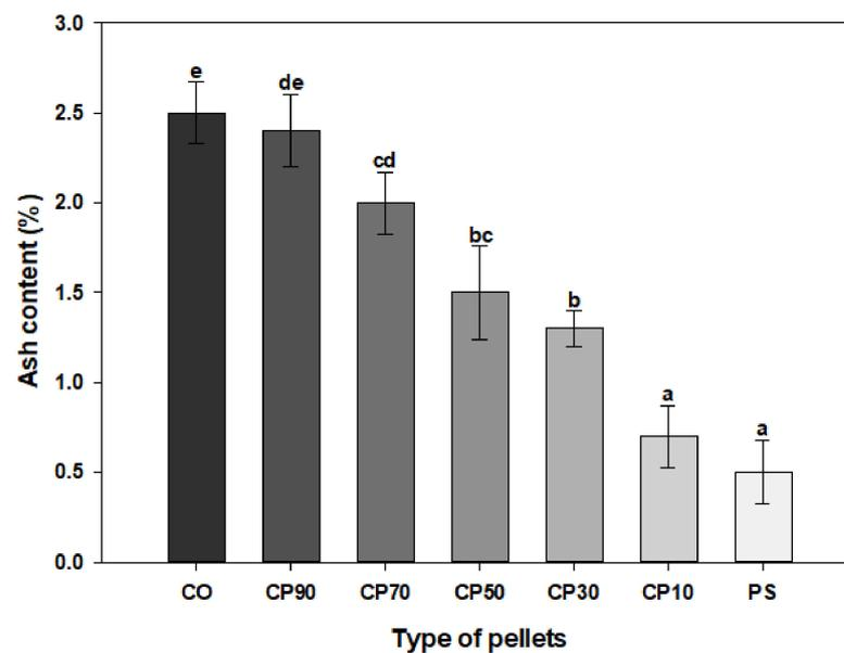
**Figure 8.** Ash content of pellets according to SCG blending ratio. Each point is the mean of three repeated measurements and is the mean  $\pm$  standard deviation. The means with different letters (a–e) above the bars indicate significant differences based on Tukey’s HSD test ( $p < 0.05$ ).
