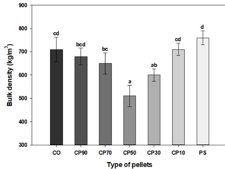
**Figure 4.** Bulk density of pellets according to SCG blending ratio. Each point is the mean of three repeated measurements and is the mean  $\pm$  standard deviation. The means with different letters (a–d) above the bars indicate significant differences based on Tukey’s HSD test ( $p < 0.05$ ).
