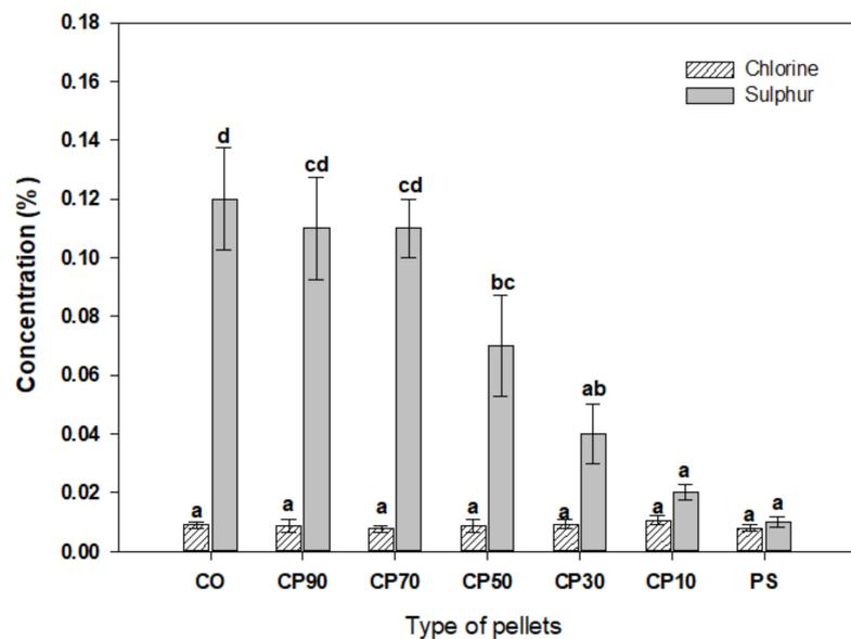
**Figure 9.** S and Cl concentrations of pellets according to SCG blending ratio. Each point is the mean of three repeated measurements and is the mean  $\pm$  standard deviation. The means with different letters (a–d) above the bars indicate significant differences based on Tukey’s HSD test ( $p < 0.05$ ).
