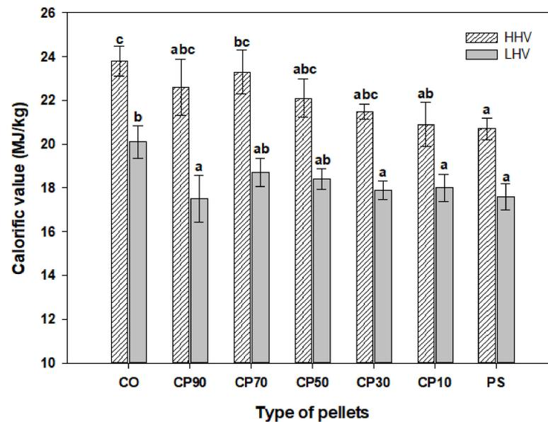
**Figure 7.** Pellet heating value according to SCG blending ratio. Each point is the mean of three repeated measurements and is the mean  $\pm$  standard deviation. The means with different letters (a–c) above the bars indicate significant differences based on Tukey's HSD test ( $p < 0.05$ ).
