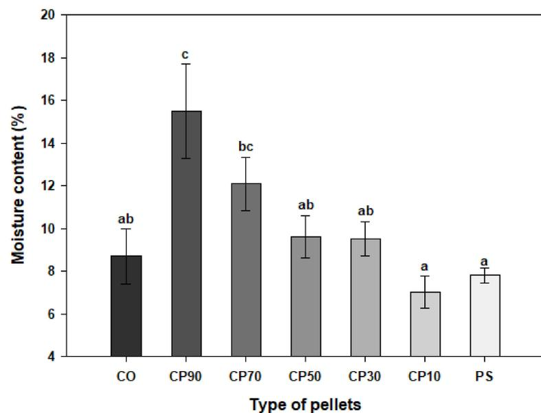
**Figure 5.** Pellet moisture content according to SCG blending ratio. Each point is the mean of three repeated measurements and is the mean  $\pm$  standard deviation. The means with different letters (a–c) above the bars indicate significant differences based on Tukey’s HSD test ( $p < 0.05$ ).
