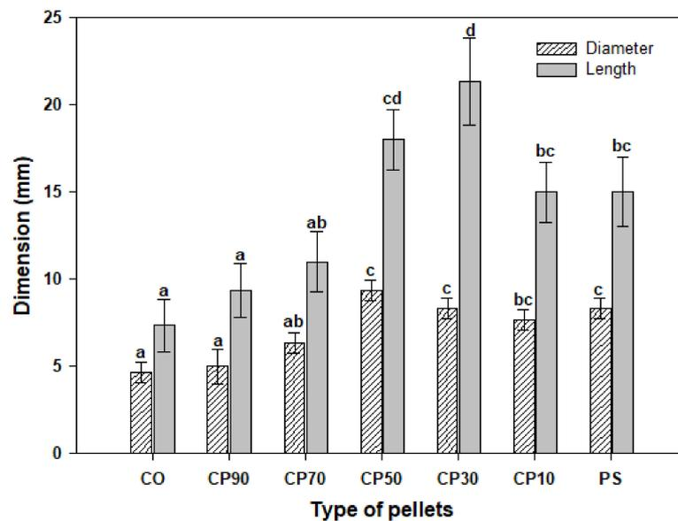
**Figure 2.** Pellet size according to SCG blending ratio. Each point is the mean of three repeated measurements and is the mean  $\pm$  standard deviation. The means with different letters (a–d) above the bars indicate significant differences based on Tukey’s honest significant difference (HSD) test ( $p < 0.05$ ).
