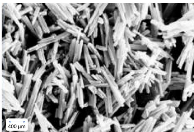
**Figure 8.** SEM image of  $\alpha$ -MnO<sub>2</sub> nanorod. Reprinted with permission from [30]. Copyright 2015 American Chemical Society.
