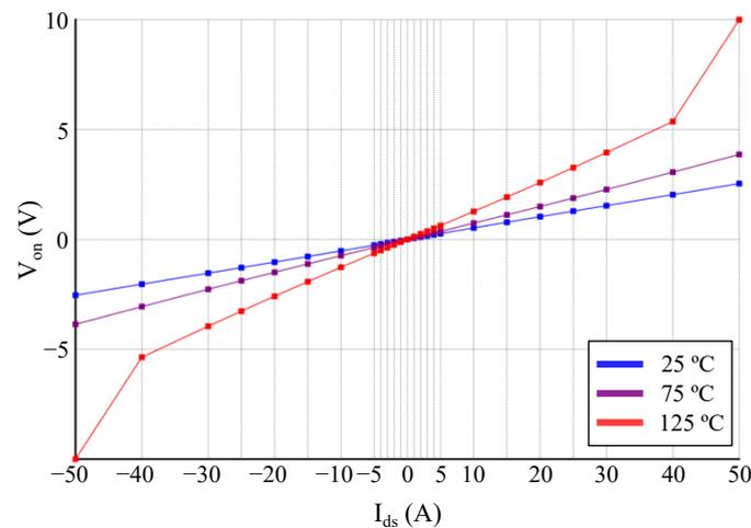
Figure 9. GaN e-HEMT conduction losses look-up table.
