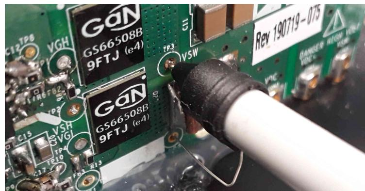
Figure 17. Drain-source voltage measurement technique.
