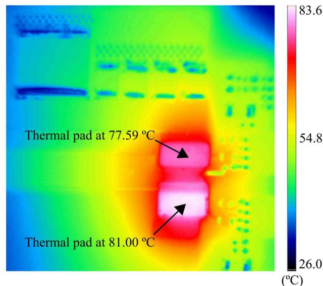
**Figure 21.** Thermogram of the top-side cooled converter without heatsink.
