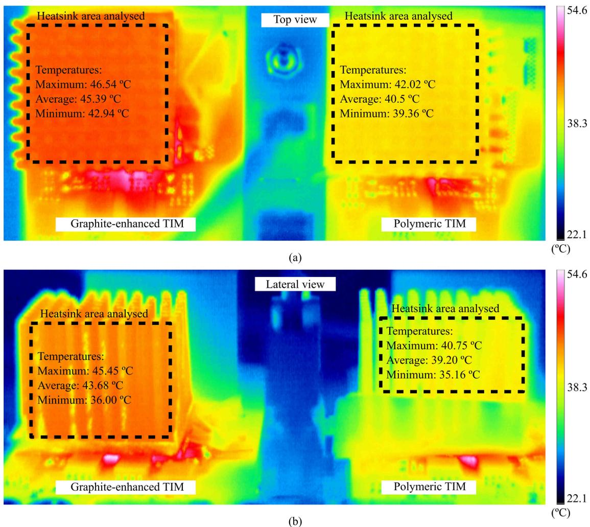
**Figure 23.** Thermal images of the top-side cooled converter: (a) top view and (b) lateral view.
