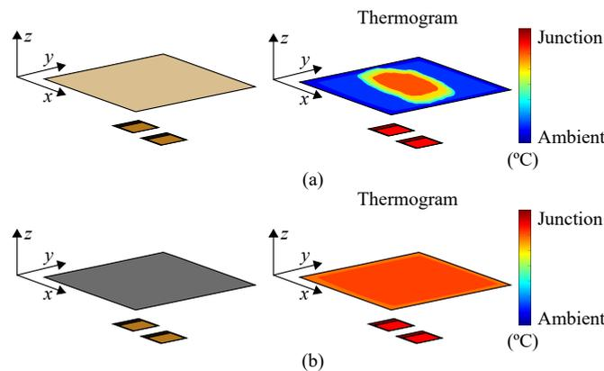
**Figure 3.** Representation of heat flow through: (a) a polymeric TIM; and (b) a graphite-enhanced TIM.
