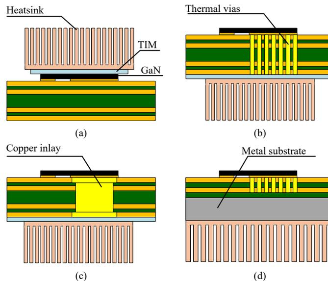
**Figure 2.** Heat dissipation methods: (a) top-side cooled, (b) bottom-side cooled with vias, (c) bottom-side cooled with copper inlay, and (d) insulated metal substrate.
