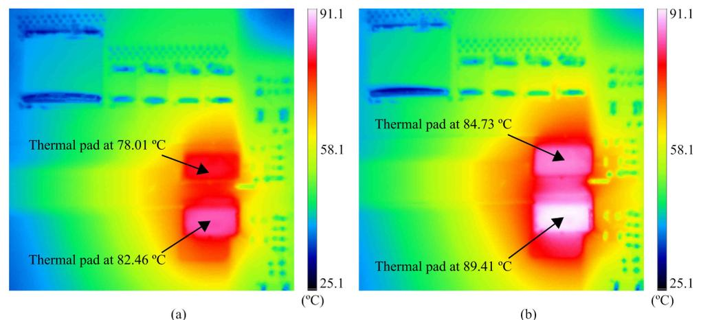
**Figure 19.** Thermal images of the GaN-based converter using different deadtimes: (a) 40 ns and (b) 100 ns.
