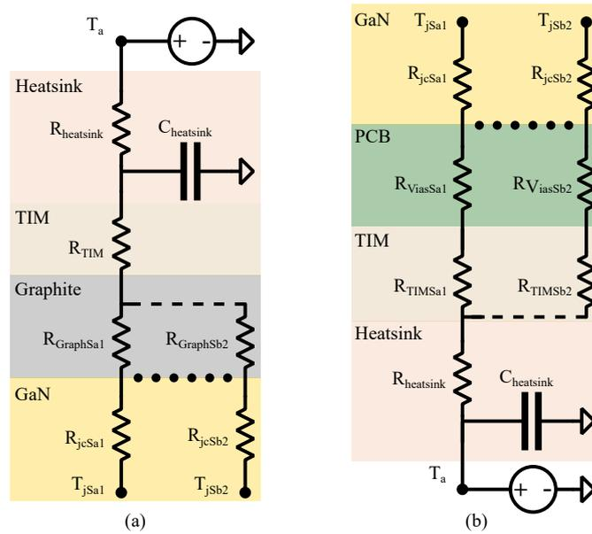
Figure 5. Thermal model of a converter with: (a) top-side cooled GaN e-HEMTs; and (b) bottom-side cooled GaN e-HEMTs.
