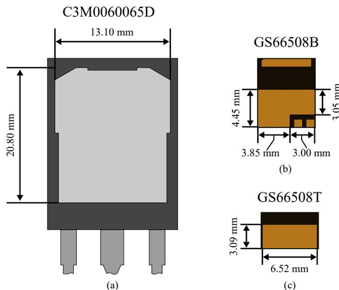
**Figure 1.** Size comparison between: (a) SiC MOSFET; (b) bottom-side cooled GaN e-HEMT; and (c) top-side cooled GaN e-HEMT. Thermal pad measurements are shown. The transistors are drawn to scale with each other.
