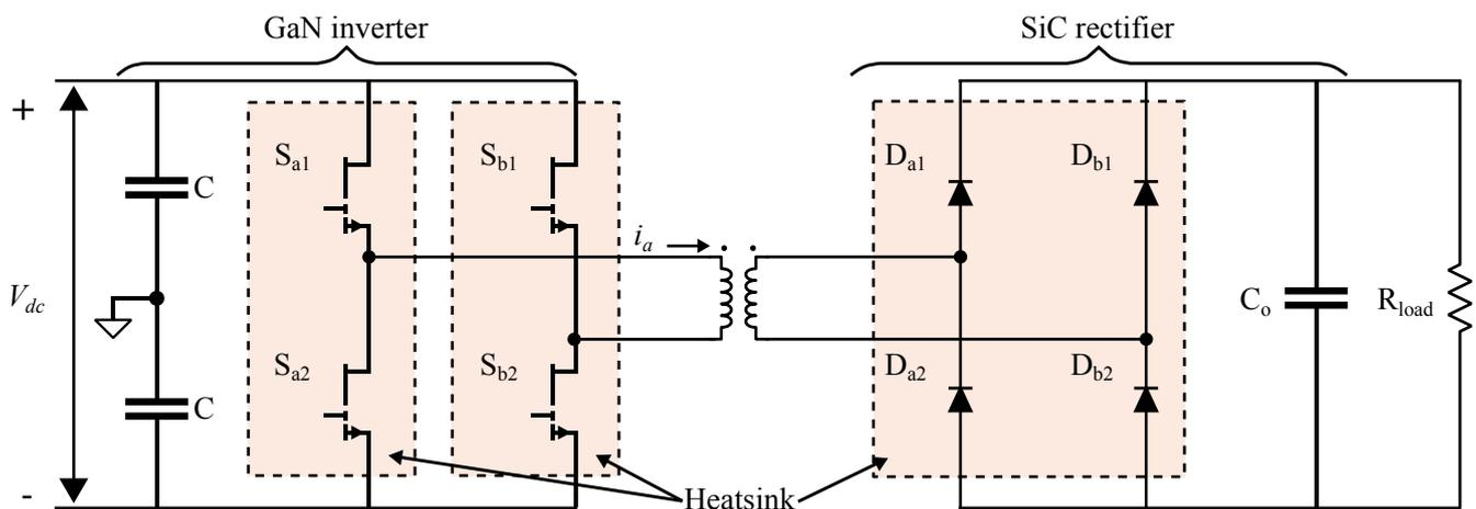
Figure 10. Schematic of the power converter. The heatsinks are drawn with dashed lines.
