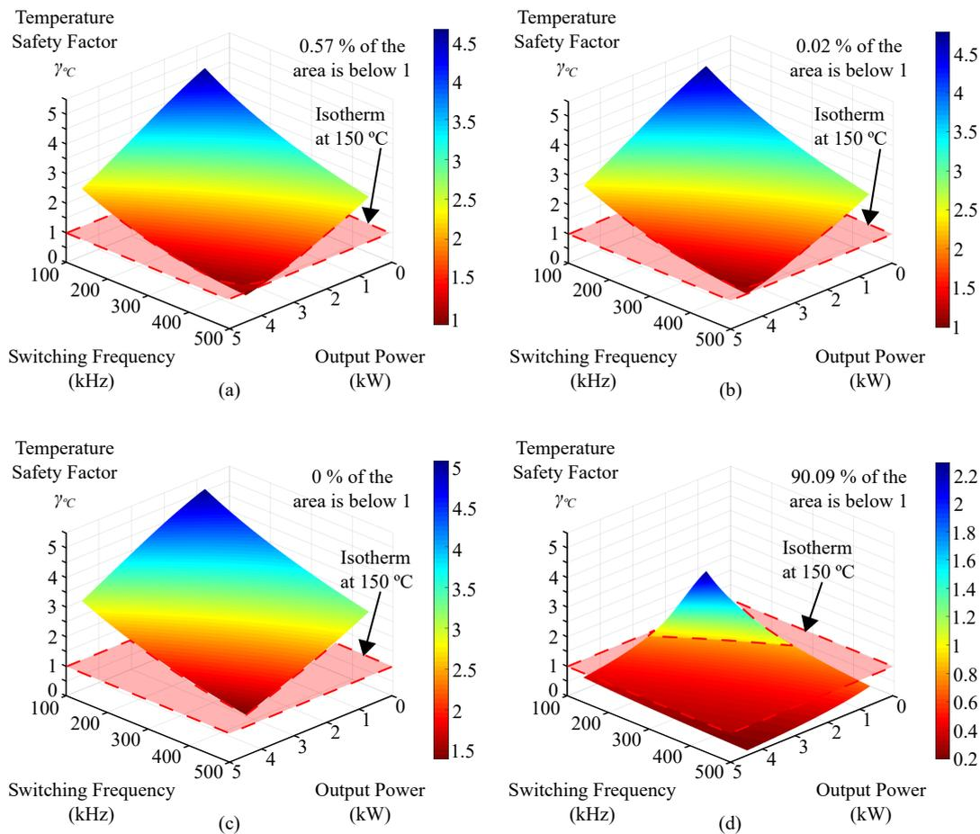
**Figure 11.** Junction temperature safety factor: (a) bottom-side cooled converter; (b) top-side cooled converter with graphite-enhanced and polymeric TIMs; (c) top-side cooled converter with a graphite-enhanced TIM; and (d) top-side cooled converter with a polymeric TIM.
