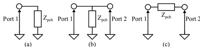
**Figure 13.** Techniques for measuring S parameters: (a) 1-port reflection; (b) 2-port shunt-thru; and (c) 2-port series-thru.
