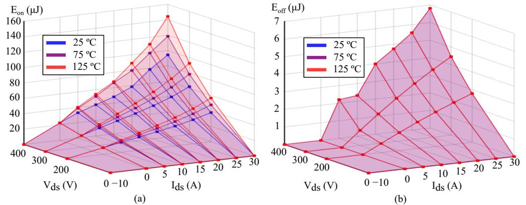
Figure 8. GaN e-HEMTs look-up tables: (a) turn-on and (b) turn-off losses.
