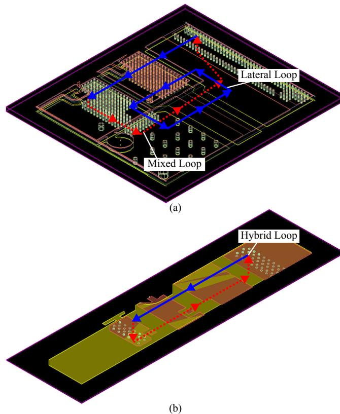
**Figure 14.** Power converters modelled in ADS: (a) bottom-side cooled converter; and (b) top-side cooled converter. The top-side currents are drawn using blue lines. The currents that flow through inner layers are drawn using red dashed lines.
