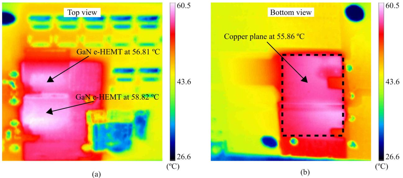
**Figure 20.** Thermogram of the bottom-side cooled converter without heatsink: (a) bottom view; and (b) top view.
