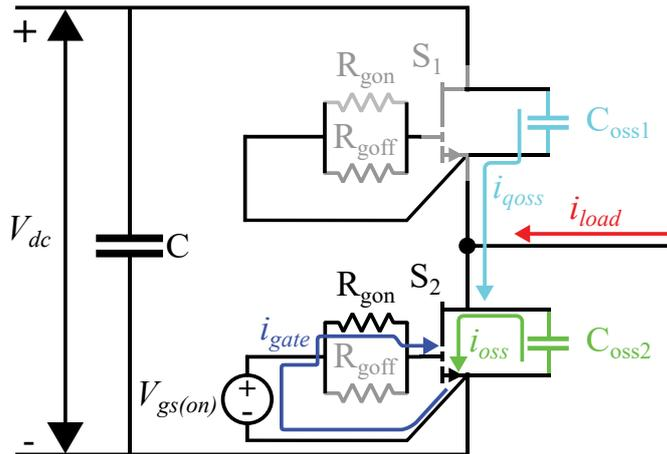
Figure 7. Half-bridge electrical circuit the turn-on process.
