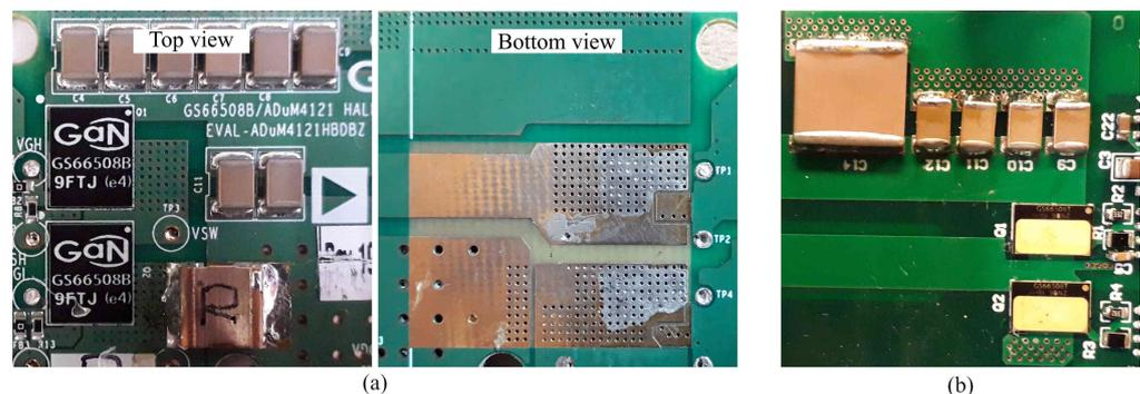
Figure 16. View of the GaN-based power converters: (a) bottom-side cooled converter; and (b) top-side cooled converter.
