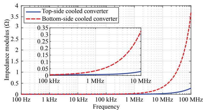
Figure 15. PCB impedances obtained from an electromagnetic simulation.
