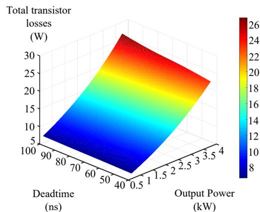
**Figure 12.** Total transistor losses as a function of deadtime and output power.
