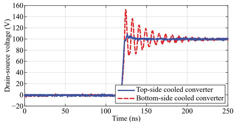
Figure 18. Comparison between the experimental drain-source voltages of the studied converters.
