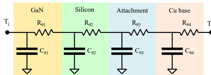
**Figure 4.** Equivalent thermal model of a GaN e-HEMT.
