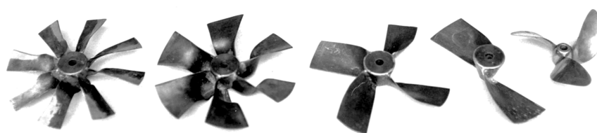
Figure 6. Experimental impellers with fixed blades. Source: [5].
