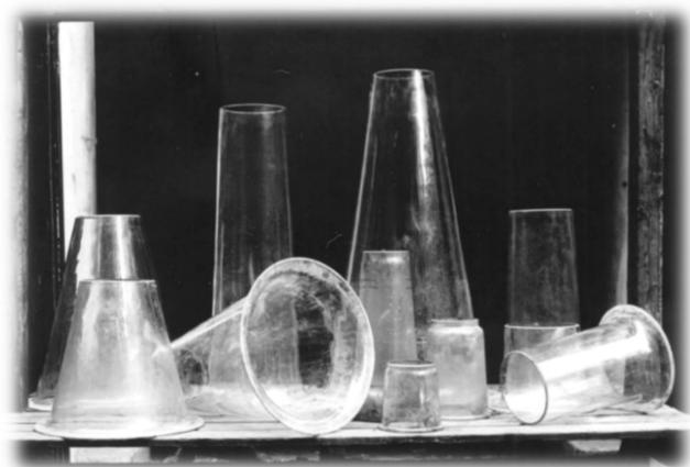
Figure 11. Glass draft tubes used in the experiments. Source: [5].
