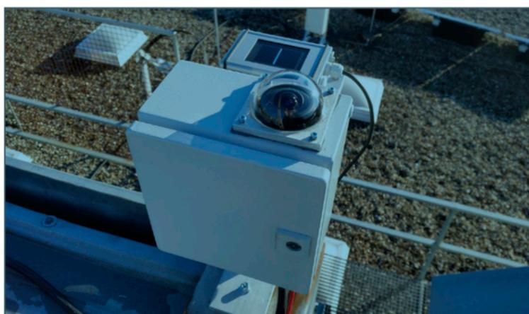
**Figure 1.** The ground-based camera sensor system positioned at Offenburg University.
