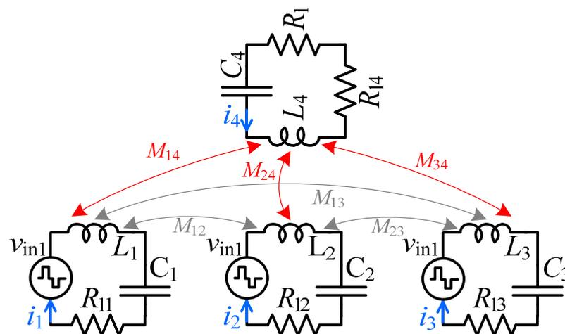
Figure 5. Simplified model of the multicore transmitter solution.
