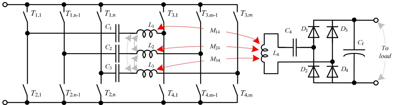
Figure 4. Inductive power transfer topology with three transmitters.
