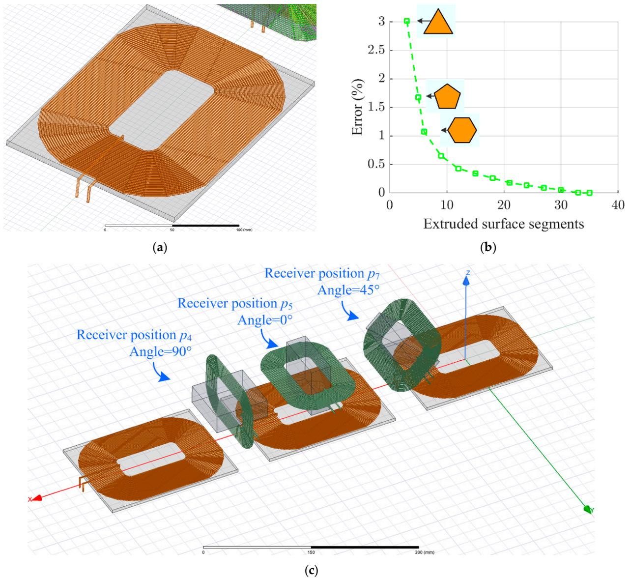
**Figure 6.** Simulation model for the FEM analysis: (a) transmitter coils ( $L_1, L_2, L_3$ ) design, (b) simulation error of the coil parameters for different extruded surface segments and (c) different positions of the receiver along the track.
