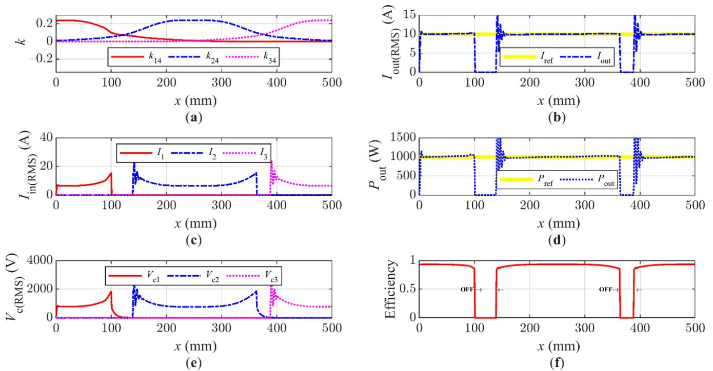
**Figure 9.** Second solution: (a) coupling coefficients  $k_{14}$ ,  $k_{24}$  and  $k_{34}$ ; (b) output current  $I_{out(RMS)}$ ; (c) input currents  $i_{1(RMS)}$ ,  $i_{2(RMS)}$  and  $i_{3(RMS)}$ ; (d) output power  $P_{out(RMS)}$ ; (e) voltages on the primary side capacitor  $v_{c1(RMS)}$ ,  $v_{c2(RMS)}$  and  $v_{c3(RMS)}$ ; (f) system efficiency.
