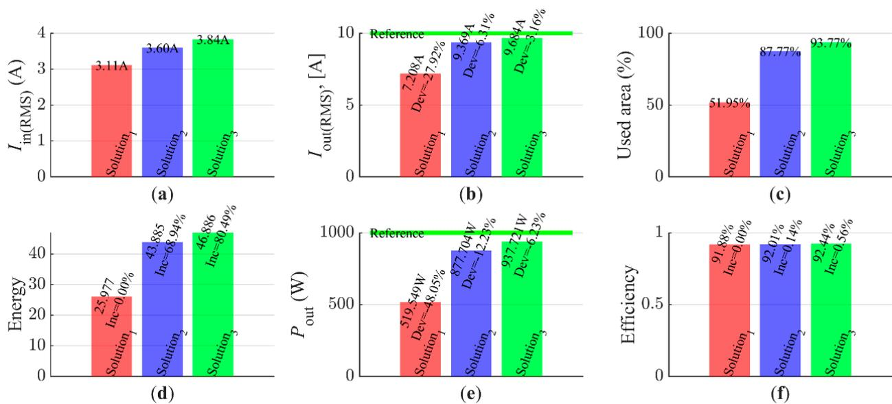
**Figure 14.** Comparison of three solutions: (a) input current  $I_{in(RMS)}$ ; (b) output current  $I_{out(RMS)}$ ; (c) used track area; (d) transmitted energy  $E$ ; (e) transmitted power  $P_{out(RMS)}$ ; (f) system efficiency.
