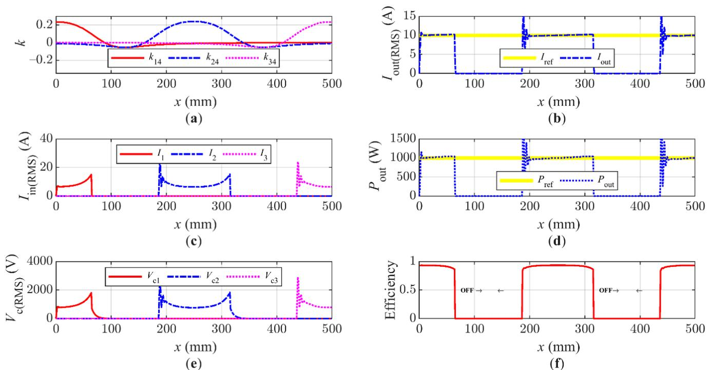
**Figure 8.** First solution: (a) coupling coefficients  $k_{14}$ ,  $k_{24}$  and  $k_{34}$ ; (b) output current  $I_{out(RMS)}$ ; (c) input currents  $i_{1(RMS)}$ ,  $i_{2(RMS)}$  and  $i_{3(RMS)}$ ; (d) output power  $P_{out(RMS)}$ ; (e) voltages on the primary side capacitor  $v_{c1(RMS)}$ ,  $v_{c2(RMS)}$  and  $v_{c3(RMS)}$ ; (f) system efficiency.
