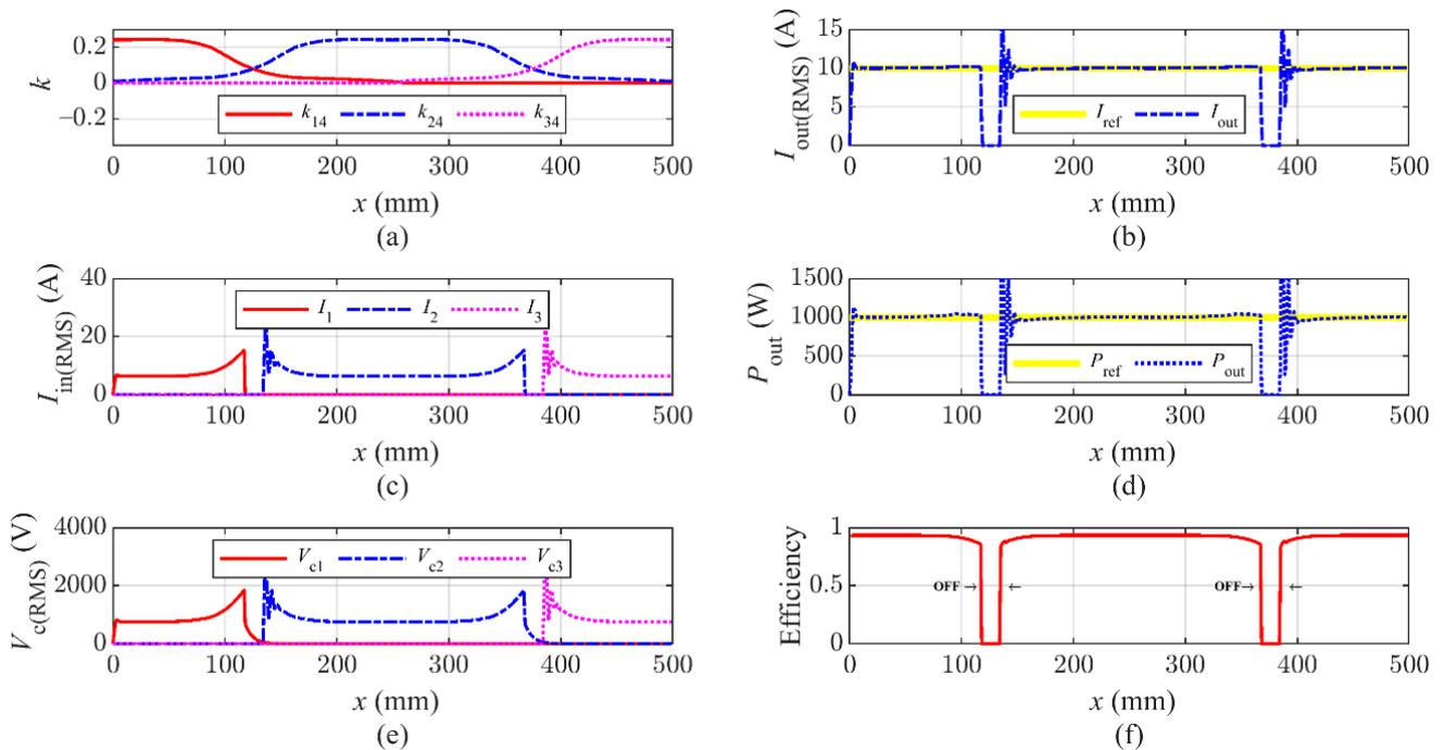
Figure 12. Third solution: (a) coupling coefficients  $k_{14}$ ,  $k_{24}$  and  $k_{34}$ ; (b) output current  $I_{out(RMS)}$ ; (c) input currents  $i_1(RMS)$ ,  $i_2(RMS)$  and  $i_3(RMS)$ ; (d) output power  $P_{out(RMS)}$ ; (e) voltages on a primary side capacitor  $v_{c1(RMS)}$ ,  $v_{c2(RMS)}$  and  $v_{c3(RMS)}$ ; (f) system efficiency.
