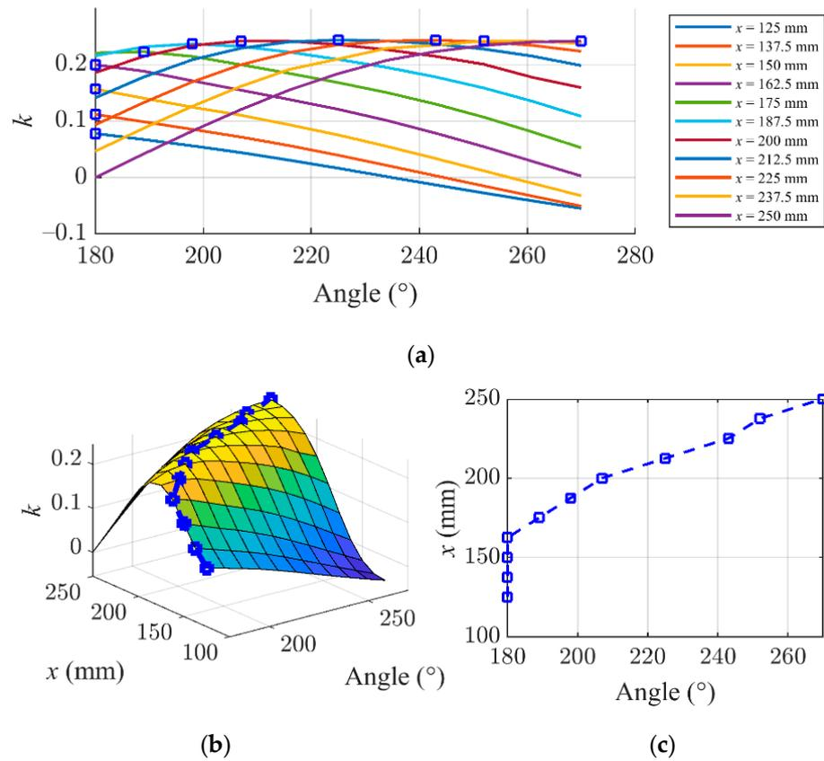
Figure 11. Simulation results of optimal movement trajectory: (a) coupling coefficients for different receiver coil angles, (b) surface with the optimal trajectory of movement and (c) optimal trajectory.
