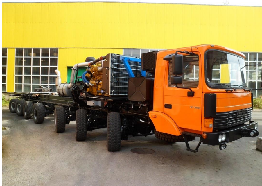
Figure 1. The truck with one chassis and two engines.
