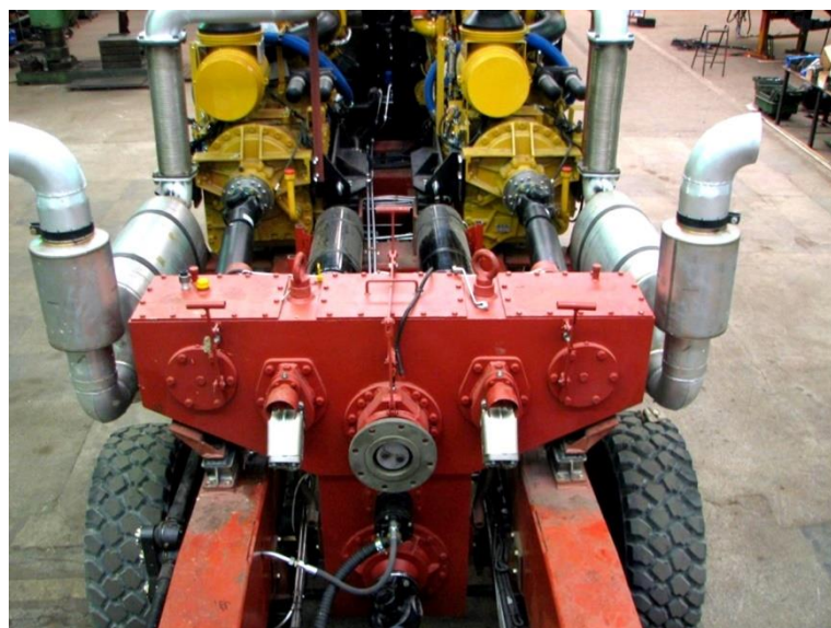
Figure 2. The adder and distribution box.
