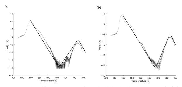
Figure 10. Regression lines of characteristic temperature for grape branch (a) and perilla (b) at a heating rate of 7.5 °C/min.
