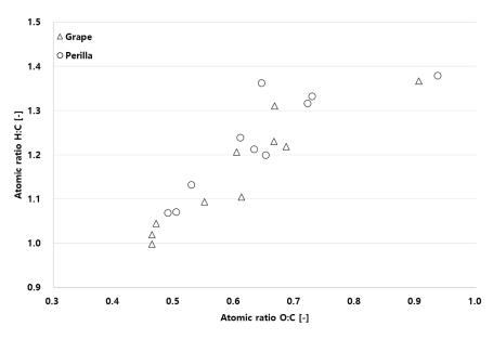
Figure 5. Van Krevelen diagram of torrefied grape and perilla.
