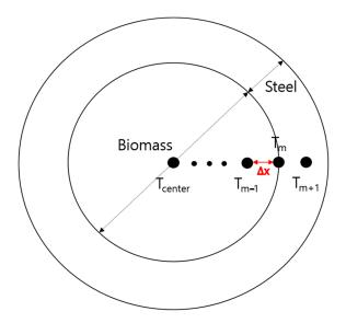
Figure 3. Finite element analysis to predict each node temperature in prototype capsule.
