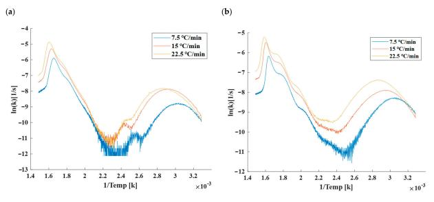
Figure 9. Arrhenius plot of TGA data measured at different heating rates of grape branch (a) and perilla (b).
