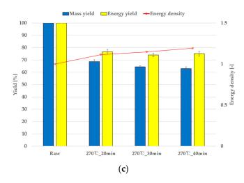
**Figure 6.** Grape mass and energy yields and energy density according to torrefaction process time and temperature. (**a**) At 200 °C, (**b**) at 230 °C, and (**c**) at 270 °C.
