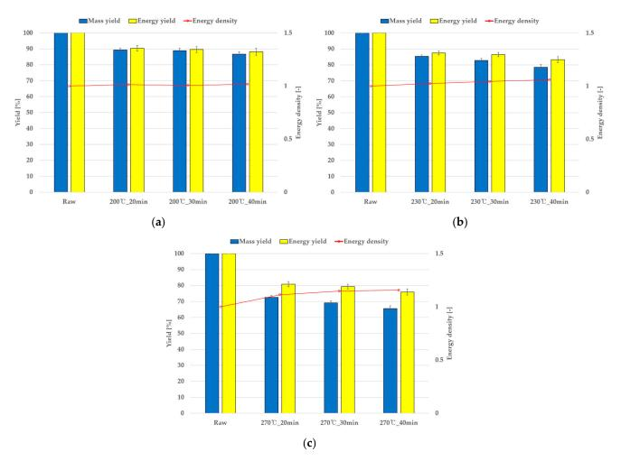
**Figure 7.** Perilla mass and energy yields and energy density according to torrefaction process time and temperature. (**a**) At 200  $^{\circ}$ C, (**b**) at 230  $^{\circ}$ C, and (**c**) at 270  $^{\circ}$ C.
