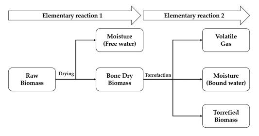
Figure 4. Thermochemical conversion of biomass [2].
