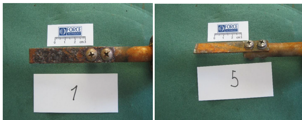
(a) Steel coupon exposed for 5 months
