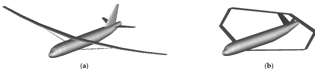
Figure 3. (a) Strut-braced and (b) box wing configurations designed in OpenVSP based on A320 design (adapted from [24]).
