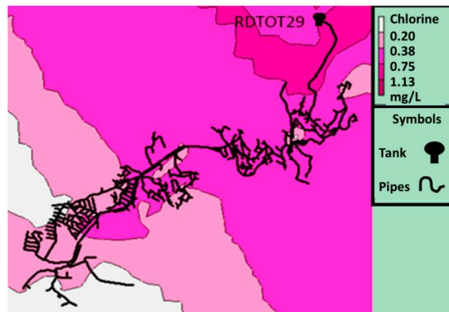
Figure 4. Contour plot of chlorine distribution in the initial condition from WDN “SF812”.
