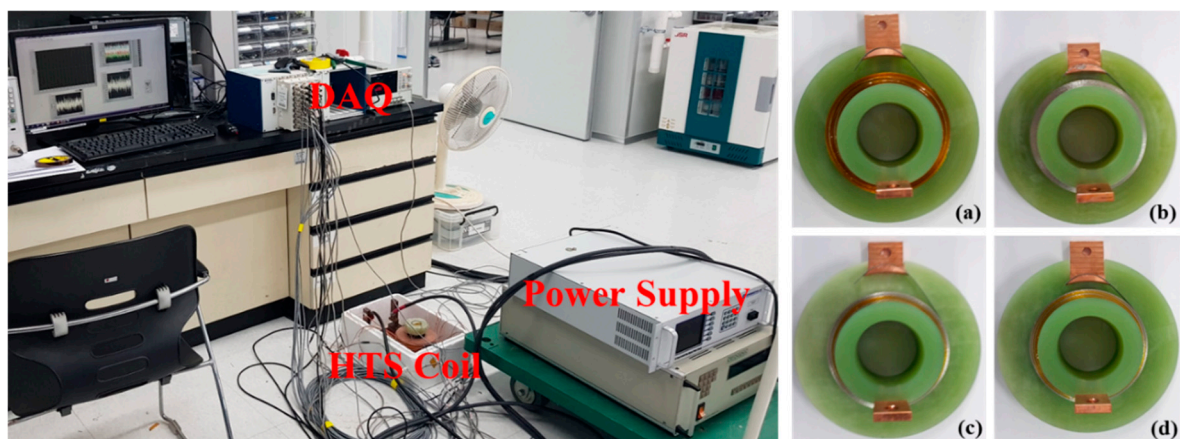
Figure 1. Experimental setup and HTS coils for charging/discharging tests: (a) Coil I, (b) Coil II, (c) Coil III, and (d) Coil IV.
