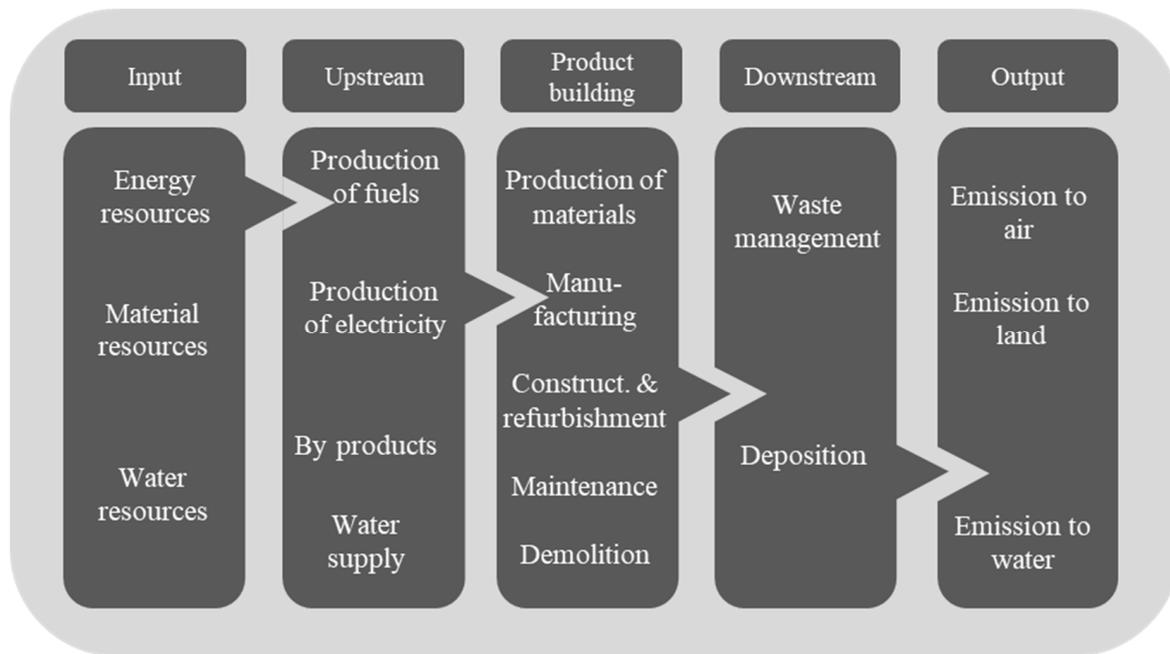
**Figure 4.** Cradle-to-grave scheme for evaluating the ecological impact of a technology (based on [41–43]).
