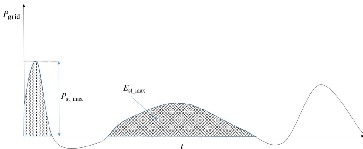
**Figure 7.** Qualitative visualization of energy storage systems sizing approach.
