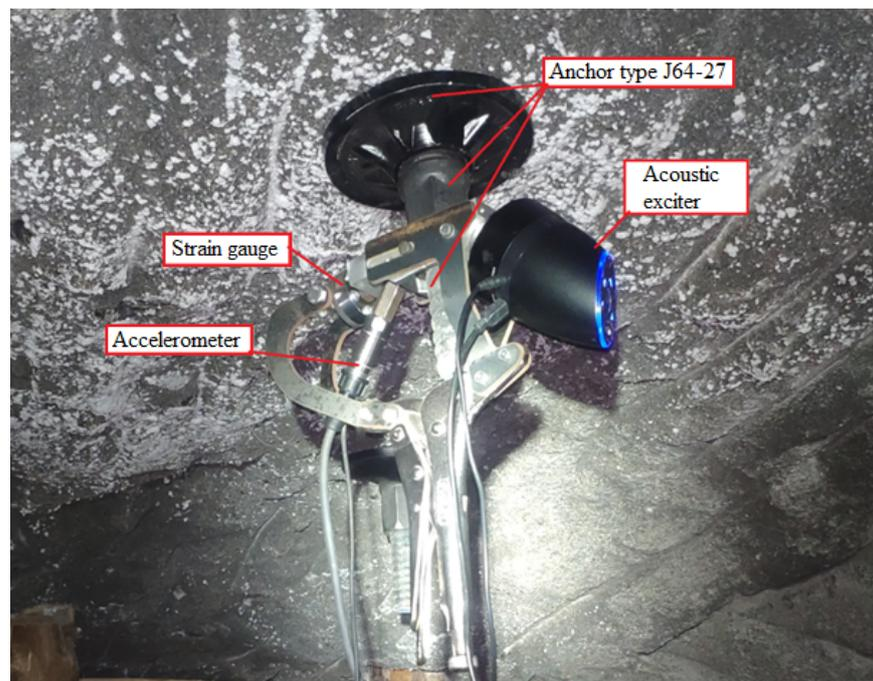
**Figure 11.** Testing fixture used during testing.
