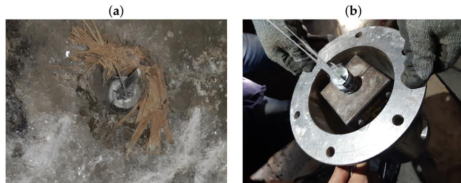
Figure 17. Anchor K3 (Vernier) after breaking using destructive test: (a) roof anchor; (b) broken anchor.
