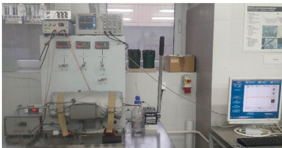
**Figure 4.** Acoustic velocity measurement apparatus.
