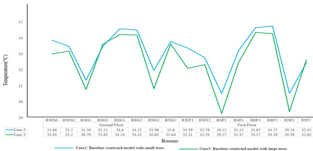
Figure 26. Comparison of air temperature for Case 2 and Case 3 in each room.
